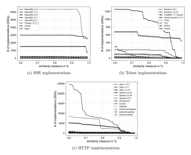
Figure 4.2: Similarity of SSH, Telnet and HTTP implementations in the Internet-wide scan based on their responses to our probes. Results are based on the latest scans for each protocol.
