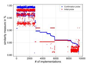
(b) Result confirmation: For all of the fingerprinted honeypots the cosine similarity score for both, the initial probe and the confirmation probe is 0.90 or higher.
