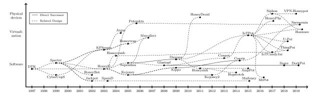
Figure 2.1: Evolution of server honeypots from 1997 to 2019. Solid lines signify a direct successor. Dashed lines signify a related design, including the choice of protocol(s), emulation of specific versus generic (vulnerable) services, and purpose (monitoring, prevention, detection, response or profiling).
