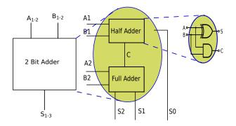
Figure 4.1: A heirarchical model of a 2-bit adder.
