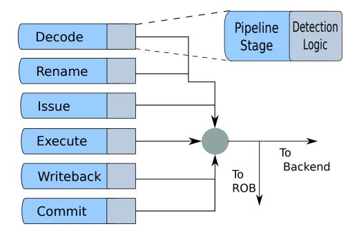
Figure 5.5: PreFix detection logic. Each component has a related detector and any trigger causes a re-execution.
