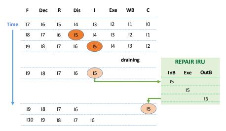
Figure 3.4: Example rerun of an instruction using REPAIR.
