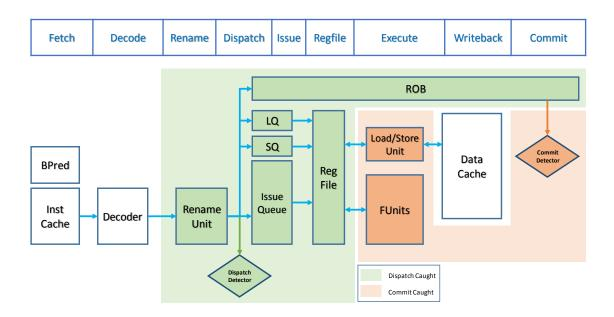
Figure 3.3: Detection stages within a core.
