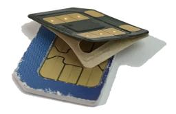
Figure 6.1: An overlay SIM (top) and a regular SIM (bottom). The top part of the overlay SIM can be peeled off and stuck on top of a regular SIM
