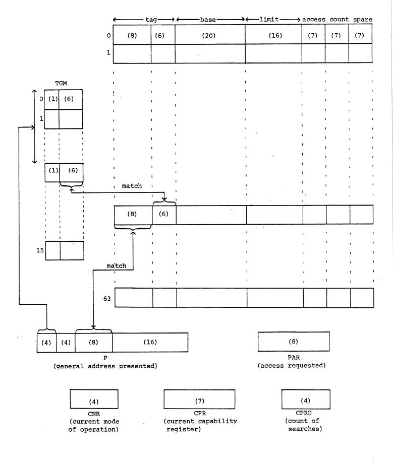
Figure 3.6 : Capability Unit layout
