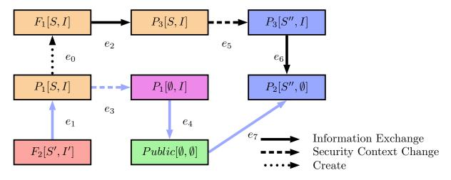
Figure 5.1: Simplified audit graph from IFC OS execution (we omit metadata for readability). Blue/pale arrows show the path to disclosure.
