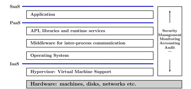
Figure 1.1: Classic cloud service provision architecture. Providers (offer and) manage services below the associated (blue) line, and tenants those above [Pasquier et al. 2014a].
