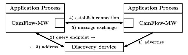
Figure 4.1: CamFlow-MW overview
