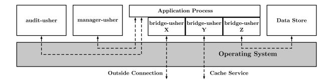
Figure 3.5: Ushers and an application process.
