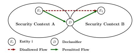
Figure 1.3: Transferring data across security contexts through a Declassifier (or Endorser, not shown).
