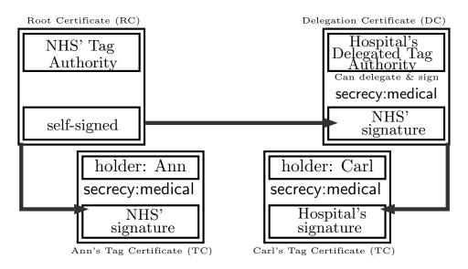
Figure 4.3: Two (simplified) Tag Certificates representing the same tag (same name, valid signature chain with the same root)
