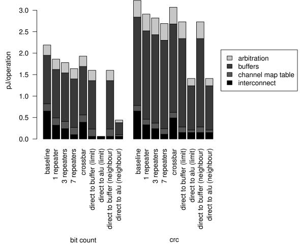
**Figure 6.22:** Energy comparison for different core-to-core interconnect options. *limit*: direct links between arbitrary cores; *neighbour*: direct links between adjacent cores only.
