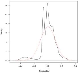
(c) A poor model which needs refinement. The extra peaks indicate that important information is not being included in the model.
