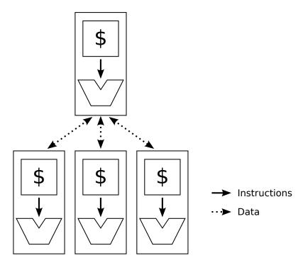
**Figure 6.9:** Worker farm execution pattern. One core is designated the *master* and is removed from the DLP group and made responsible for distributing tasks among the other cores. Workers let the master know when they would like to be issued more work.
