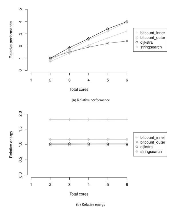
Figure 6.10: Behaviour of worker farm execution pattern relative to baseline single-core benchmark kernels.
