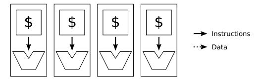
**Figure 6.1:** MIMD execution pattern. Each core independently issues instructions from its local cache, with instructions potentially coming from separate applications.
