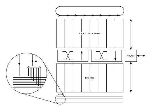
**Figure 3.8:** Sub-networks within each Loki tile. Cores and memory banks communicate with each other via fast crossbars, cores communicate with each other using buses capable of multicast, and memory banks communicate with each other using a simple ring network. A router provides links to neighbouring tiles.
