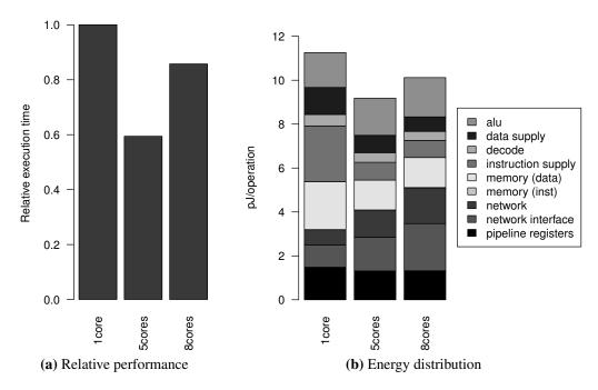
**Figure 6.16:** CRC dataflow behaviour. Instruction supply is more efficient when using the dataflow execution pattern, at a cost of increased network (buses and arbiters) and network interface (channel map table and network buffers) activity.
