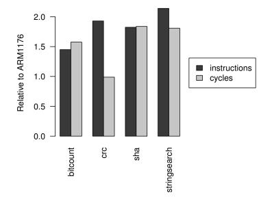
**Figure 5.11:** Comparison with ARM1176. Identical source code was used for benchmarks on the two platforms.
