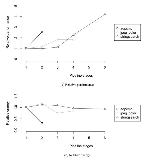
**Figure 6.13:** Relative energy and performance of task-level pipelining for a selection of MiBench kernels. All figures are relative to a single-core baseline implementation.
