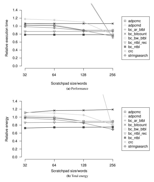
Figure 5.6: Behaviour of various sizes of scratchpad, relative to no scratchpad at all. All implementations are accessible within a single clock cycle.
