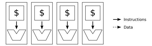
**Figure 6.2:** DLP execution pattern. Each core independently issues instructions from the same application from its local cache.
