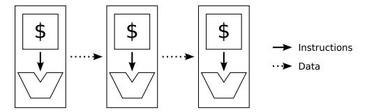
**Figure 6.12:** Task-level pipeline execution pattern. Each core performs an independent processing task on the received data, and sends the result on to the next core.
