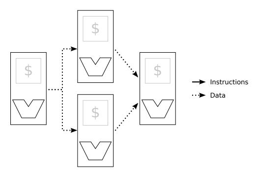
**Figure 6.14:** Dataflow execution pattern. Each core is capable of receiving up to two operands from the network, and sending its result to any subset of cores on the same tile. When executing only a single instruction on a core, it does not need to be issued repeatedly, and the entire front end of the pipeline can be power gated.
