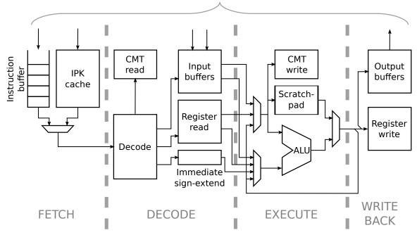
Figure 3.2: Loki pipeline block diagram.
