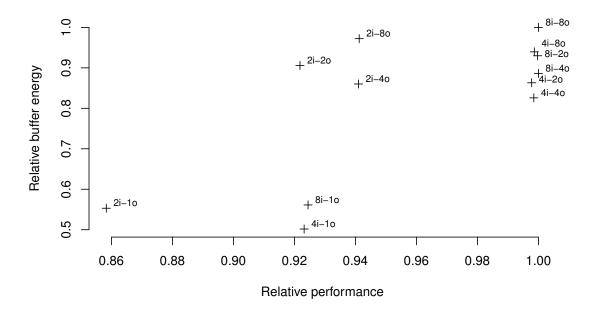
**Figure 6.21:** Network buffer design space exploration. Each point is labelled with the number of entries in the input and output buffers of each core and memory bank. Figures are relative to the 8i-80 implementation.
