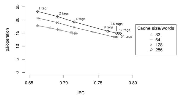
**Figure 5.1:** Normalised performance and energy consumption for different instruction packet cache sizes and numbers of tags. Tag counts start at 1 at the left of the graph and double with each step towards the right. The 256-word caches do not meet the timing constraints, and are presented for comparison only.
