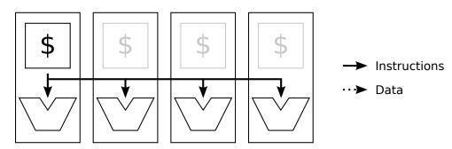
**Figure 6.7:** DLP execution pattern with instruction sharing. One core is responsible for issuing instructions to all others, mimicking SIMD architectures and reducing the cost of instruction supply. This core can change during execution to allow use of multiple L0 caches.
