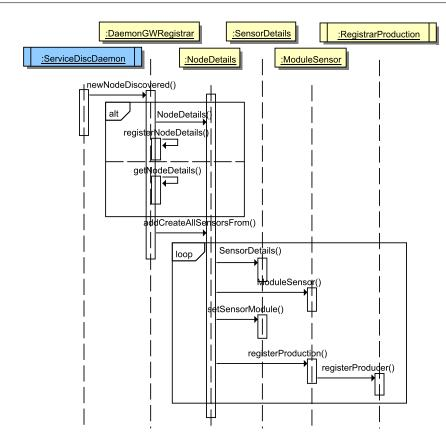
Figure 6.3 - Creation of node and sensor details
