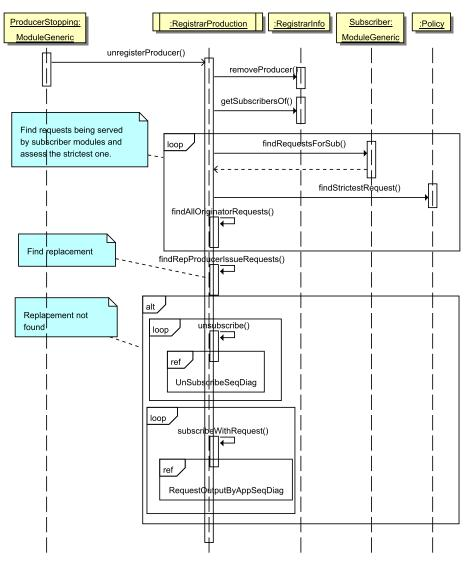
Figure 5.8 – Producer un-registering
