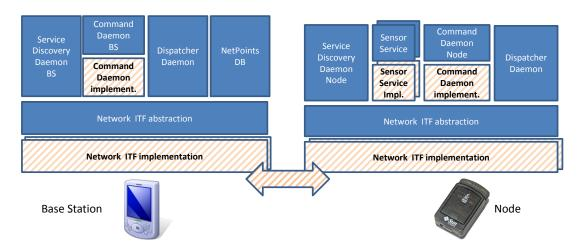
Figure 3.3 - Middleware components on the BS and node
