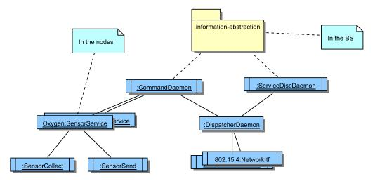
Figure 3.6 – Hardware abstraction active components
