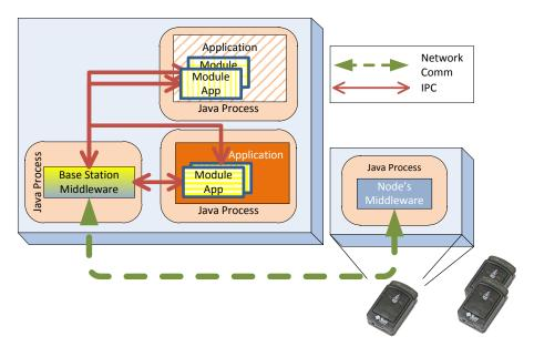
**Figure 6.6** – Communication within and in/out of BS (note that IPCs are not implemented)
