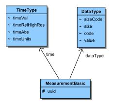
Figure 3.8 – Measure data structure and data type
