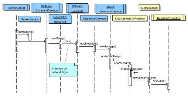
Figure 6.4 – Data new value from Sensor
