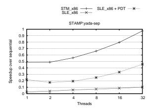
Figure 6.11: Performance of Yada after data structure decomposition
