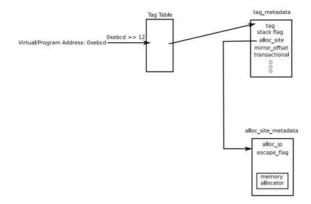
Figure 6.5: Extended tag metadata for adaptivity
