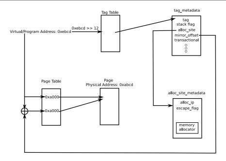
Figure 6.6: Extended tag metadata with mirror mappings
