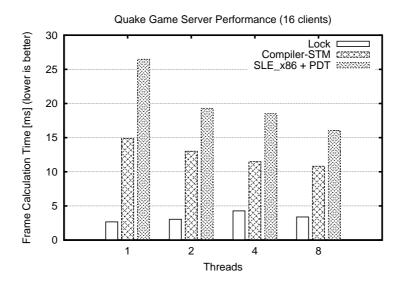
Figure 7.7: Quake using different implementations of critical sections (older Xeon system)
