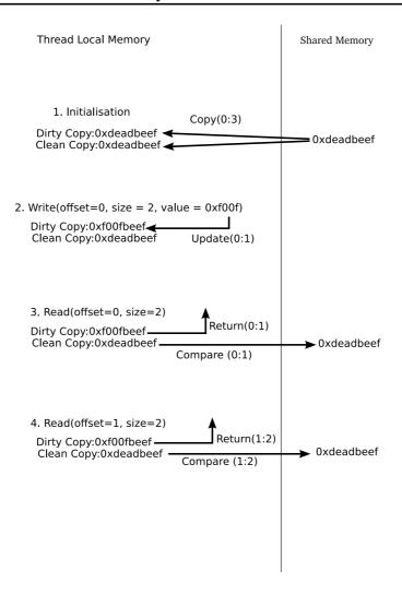
Figure 3.14: Bypassing writes to reads
