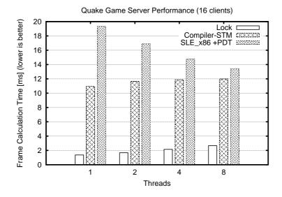
Figure 7.5: Quake using different implementations of critical sections
