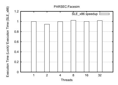
Figure 7.9: Using SLE on Facesim
