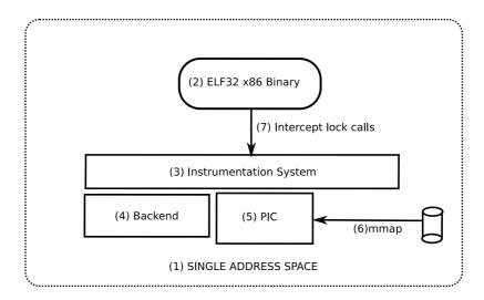
Figure 4.5: Execution in passive mode
