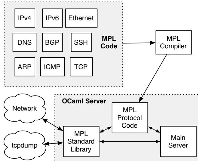
Figure 5.1: Architecture of an MPL-driven OCaml server
