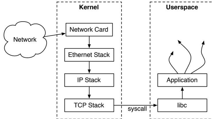
Figure 4.1: The data flow of traffic from the physical network through the kernel and finally into user-space where the buffers are sent to the application.
