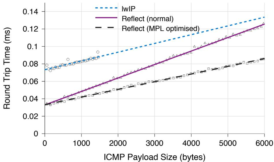
Figure 5.6: Performance of the reflecting OCaml ICMP echo server with both slow checksumming code and the MPL-optimised version
