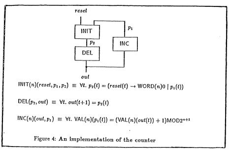
This implementation is specified at the register-transfer level, a level at which clock lines are implicit. At a lower level the delay element DEL might be implemented by a clocked D-type register with an explicit clock line; setup and hold times would then have to be represented. This lower level is not elaborated here, but it can also be modelled in predicate logic.
