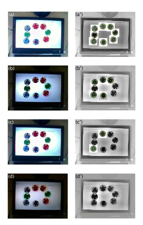
Figure A.8: Token Tracking Using State Machines and Position Matching: (a-d) as the cover is removed from the Webcam, it automatically recalibrates; (a') all 8 untracked tokens are decoded; (b') 3 tokens have repeatedly given the same code so can be tracked frame-to-frame based on their position; (c') 2 token remaining untracked; (d') all tokens tracked based on their low-resolution position.
