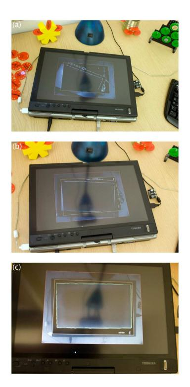
Figure A.4: Interactive Camera–Surface Calibration: (a,b) feedback as to the relative positioning of the Webcam and tablet PC guide the user to slide the tablet PC into the correct alignment; (c) all four corners of the tablet PC are within the target region – the user may proceed to system usage.
