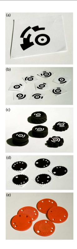
Figure 5.9: Evolution of Token Prototypes: (a) an original TRIP code; (b) my modified TRIP codes – compact, single-ringed circular codes; (c) "3D sketches" using plasticine; (d) paper mock-ups of token codes based on patterns of holes; (e) pre-production plastic prototypes constructed by drilling holes in poker chips.
