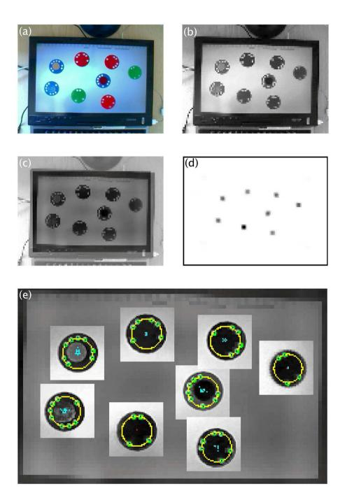
Figure A.7: Token Detection and Identification (2): (a) the high-resolution, colour Webcam image; (b) a low-resolution simple greyscale image (not used); (c) a low-resolution greyscale image based on a weighted combination of saturation and smoothed brightness; (d) response of a fast radial-symmetry 'token' detector; (e) high-resolution 'windows' around potential tokens examined for token holes. Note the harsher brightness gradient across the tablet screen compared with Figure A.6.
