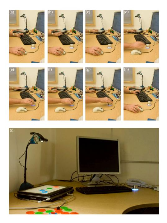
Figure 5.3: Peripheral Interaction Sequence and Interface Structure: (a) both hands in 'home' positions; (b,c) left hand lifts off keyboard and approaches token; (d) left hand nudges token as right hand lifts off the mouse; (e) right hand acquires knob as left hand retreats; (f,g) right hand rotates knob; (h) return to home position; (i) the TUI structure complements the existing monitor, mouse, and keyboard and supports peripheral interactions of the kind shown in (a-h).
