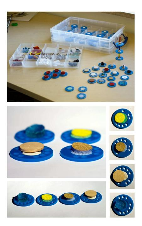
Figure 5.18: Document Token Materials and Attachment Mechanisms: The shared materials that can be attached to tokens for identification purposes can be bound to tokens via "Fuzzy-felt" backing, Velcro, white-tac, or through the use of adhesive materials such as silicone.
