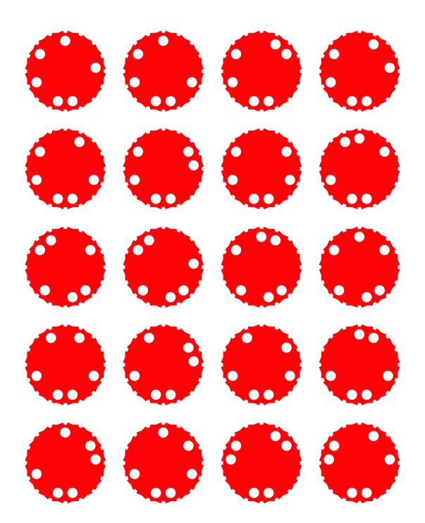
Figure A.5: Sample of Vector Graphics Token Specifications: A set of 20 matching task tokens belonging to a single user, created in Adobe Illustrator based on the output of my "token sheet generator" written in Java. Tokens were laser-cut directly from these specifications.
