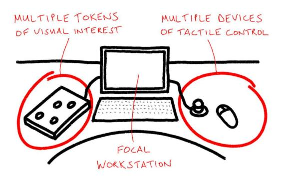
Figure 4.4: Design Sketch of a Bimanual TUI for Peripheral Interaction
