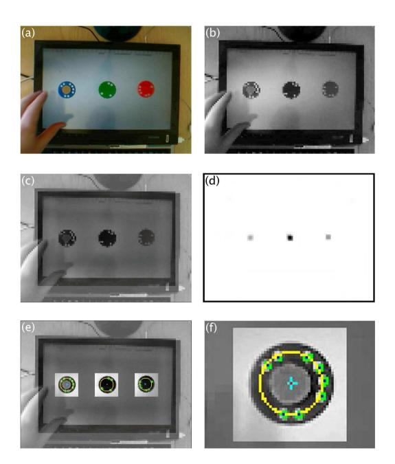
Figure A.6: Token Detection and Identification (1): (a) the high-resolution, colour Webcam image; (b) a low-resolution simple greyscale image (not used); (c) a low-resolution greyscale image based on a weighted combination of saturation and smoothed brightness; (d) response of a fast radial-symmetry "token" detector; (e) high-resolution 'windows' around potential tokens examined for token holes; (f) close-up of token decoding.
