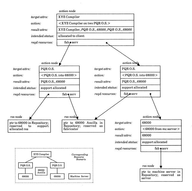
Figure 6.2. Example Blueprint for an XYZ Compiler
