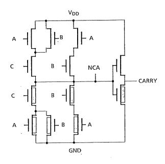
carrypart(A,B,C,NCA,CARRY) :ptrans(A,T1,1), ptrans(B,T1,1), ptrans(A,T2,1), ptrans(C,T1,NCA), ptrans(B,T2,NCA), ptrans(NCA,1,CARRY), ntrans(C,NCA,T3), ntrans(C,NCA,T4), ntrans(B,NCA,T4), ntrans(NCA,CARRY,0), ntrans(A,T3,0), ntrans(B,T3,0), ntrans(A,T4,0).
