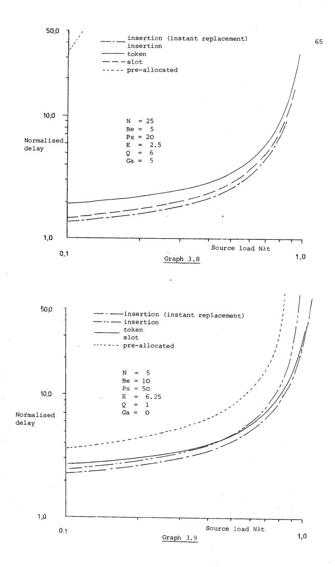
performs well under high load conditions, and since NBe = Ps all systems saturate at the same point. For low loads the slot throughput line has the same slope as the pre-allocated system (due to packets having to return to the source), whereas for p(z)N>Q the three rings are identical. The insertion replacement delay E has little effect on efficiency, and in all cases the token and insertion systems are equivalent.
