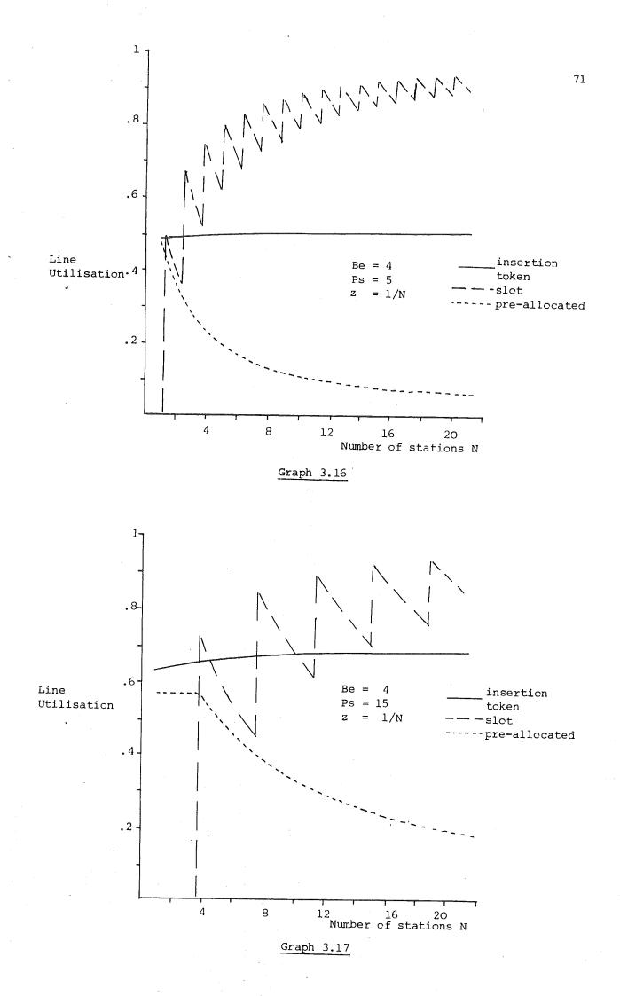
has a number of discontinuities, which have a smaller effect as N increases. It can also be seen that as N increases, the efficiency of the slot system tends to one. Graph 3.17 shows the same effect for larger packets: the efficiency of the token and insertion systems is higher, and the step function for the slot system has a greater effect.
