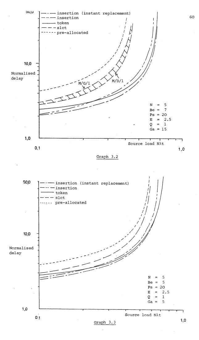
two insertion systems is small and increases with load. For low loads the token system behaves in a similar way to the slot system, and the alignment delay tends to half a ring delay. However, as load increases the token system behaves more like an insertion system (with instant replacement), and both saturate at the same point. Thus, there is a cross-over point at which the token system becomes superior to the insertion system with packet replacement time E.
