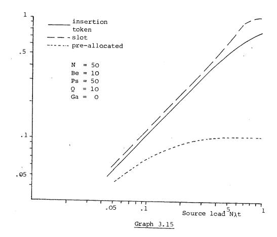
taken in reaching these points is lower for the one packet buffer model. Graph 3.15 shows a system with a large number of stations where the performance of the slot and token systems is initially similar, but at high traffic levels the slot system is better.
