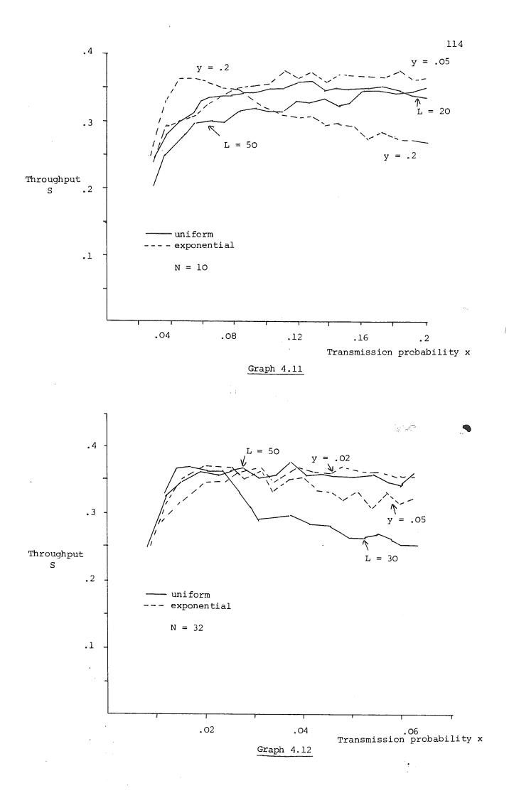
It has been shown that for a system with a small number of nodes an exponential retransmission distribution gives higher throughputs than the uniform distribution, but that as N increases, the difference between the two retransmission schemes becomes small.
