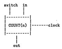
Here the input lines are switch and in, the only output line is out and the only state variable is n. The name of the device is COUNT; we write COUNT(n) (or COUNT n) to show that the behaviour (to be described) depends on n. Suppose the behaviour of COUNT is informally specified by:
