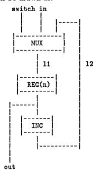
Note that MUX, REG and INC (as defined by behaviour equations above) have different line names to those in this diagram. For example, MUX was defined to have lines i1, i2 and o instead of in, 12 and 11. This illustrates our convention of using the names in diagrams to indicate renaming.
