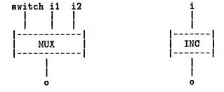
The value on the output line o of the multiplexor MUX equals the value on line i1 if the value on line switch is T, otherwise it is the value on line i2. Thus the value on the output line is given by the output equation: o=(switch->i1|i2). The behaviour of MUX is thus specified by the behaviour equation:
