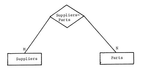
In the above example, 'Suppliers' and 'Parts' are entity sets and 'Suppliers-Parts' is a relationship set. The labels 'M' and 'N' on the arcs denote the fact that the relationship between 'Suppliers' and 'Parts' ('Suppliers-Parts') is many to many (M to N).
