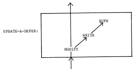
When the checking of the constraint has to be deferred a record is kept of which constraints have to be checked against the tuples written by the WRITR. The file containing these tuples is deleted after the constraints have been checked.
