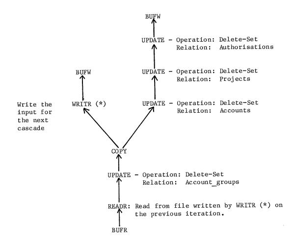
This structure executes, completes and is rebuilt until no tuples are written by WRITR (\*). For the example database the loop containing Account groups is traversed seven times.
