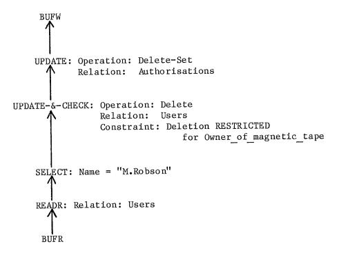
This example illustrates the use of a coroutine normally used in queries (SELECT) in an UPDATE transaction.
