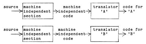
In the Algol68C system, the machine independent part of the compiler reads data (the 'initialisation file') describing the particular, machine dependent, Zcode to be produced:
