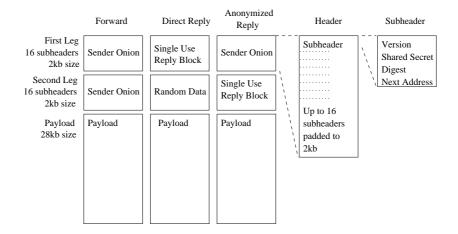
Figure 5.1: The structure of the Mixminion packet format.
