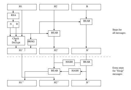
Figure 5.4: The process of decoding a Mixminion packet.
