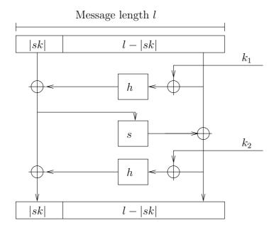
Figure 3.1: The structure of the BEAR block cipher
