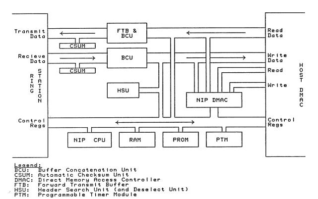
Figure 8.1 Possible High Level Interface Hardware
