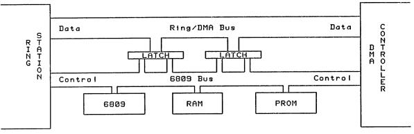
Figure 4.1 Hardware Configuration of the MACE
