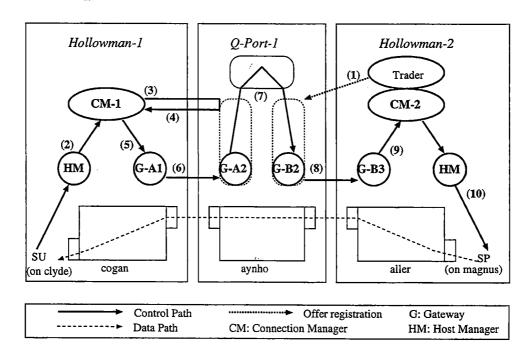
Figure 7.5: Example of Hollowman/Q.Port/Hollowman signalling
