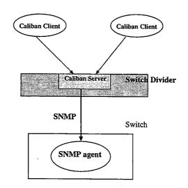
Figure 9.1: Caliban server implemented with SNMP
