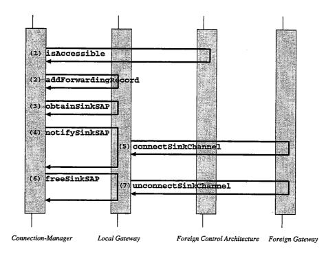
Figure 7.2: Pattern of inter-control architecture signalling
