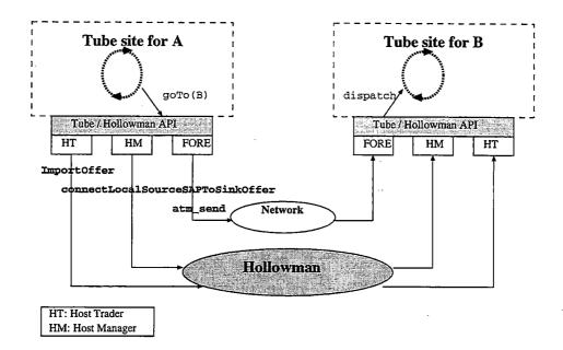
Figure 5.2: Transmitting a Tube mobile agent using the Hollowman
