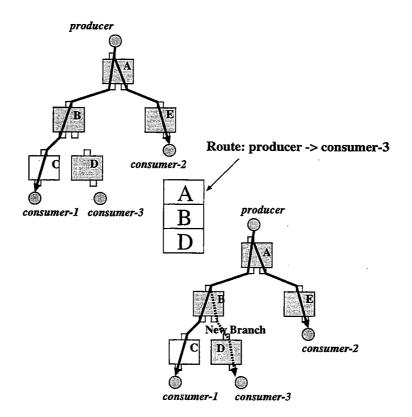
Figure 4.5: Example of multicast connection
