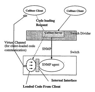
Figure 9.2: Caliban server with loaded code
