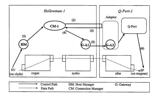
Figure 7.4: Example of Hollowman/Q.Port signalling
