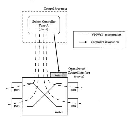
Figure 3.1: Switch control through the Ariel interface
