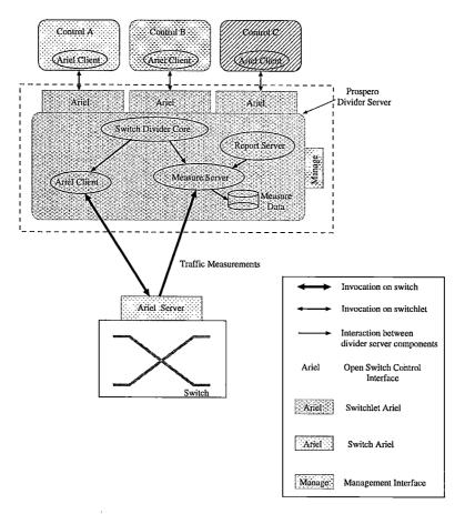
Figure 5.3: Divider Server implementation with measurement based bandwidth management
