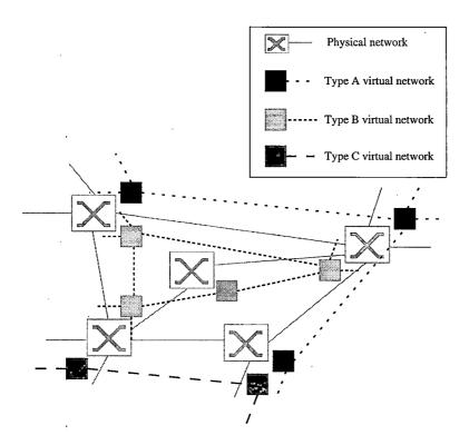
Figure 3.3: Virtual ATM networks with different control architectures
