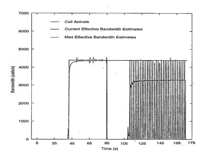
Figure 5.8: Keeping the maximum effective bandwidth for a switchlet
