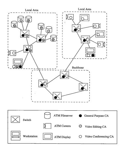
Figure 6.1: Control architectures in a physical network
