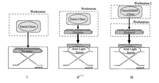
Figure 4.4: Different configurations to evaluate Prospero
