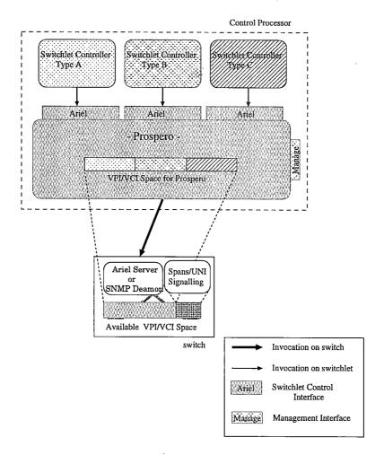
Figure 4.5: Prospero and the Bootstrap Control Architecture
