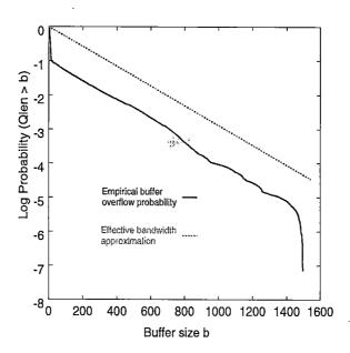
Figure 5.1: Empirical loss probability for 18 multiplexed JPEG video sources, and simple effective bandwidth approximation.
