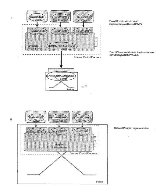
Figure 4.2: Different Ariel and Prospero implementations: (I) Divider Server on external processor, (II) Divider Server on onboard processor
