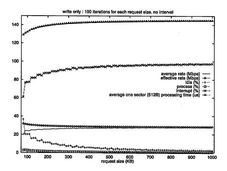
Figure 8.10: Disk Write with Increasing Request Size
