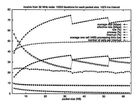
Figure 8.6: Network Receive from Fast Source
