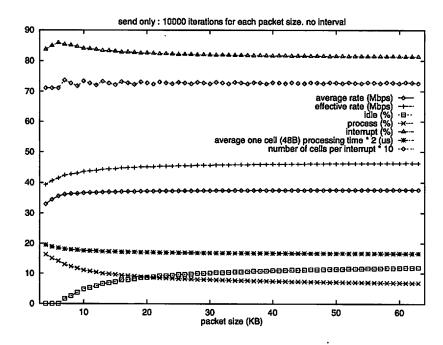
Figure 8.3: Network Send with Increasing Packet Size
