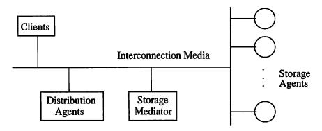
Figure 3.1: Components of the Swift Architecture
