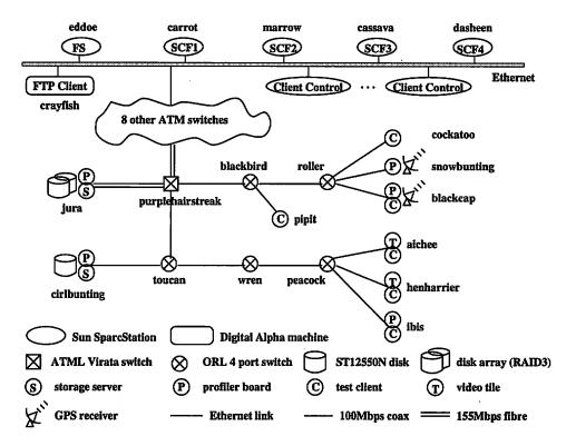
Figure 8.1: Equipment Deployment
