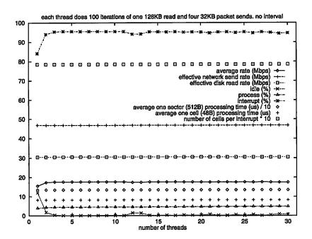
Figure 8.12: Concurrent Disk Read and Network Send
