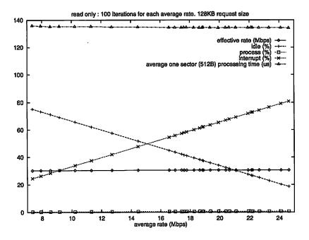
Figure 8.9: Disk Read with Increasing Average Rate
