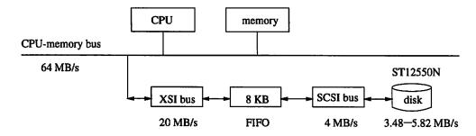
Figure 8.7: Disk Side Data Path
