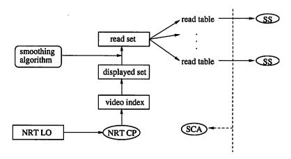
Figure 4.3: VBR Processing in the SCA for Playback
