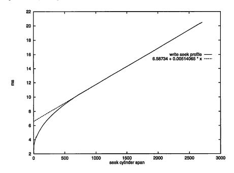
Figure 8.13: ST12550N Write Seek Time Profile and Approximation
