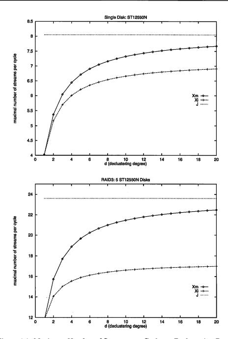
Figure 4.4: Maximum Number of Streams per Cycle vs. Declustering Degree
