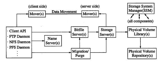
Figure 3.3: The HPSS Software Architecture
