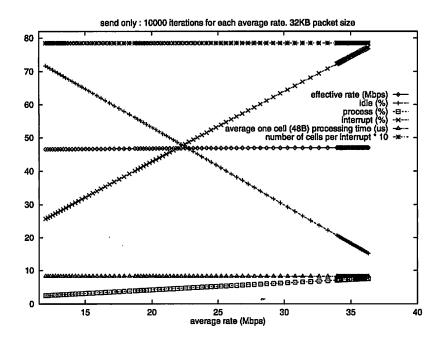
Figure 8.4: Network Send with Increasing Average Rate
