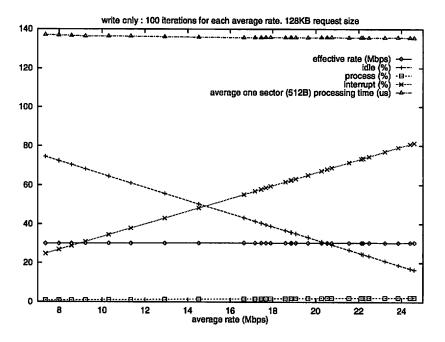
Figure 8.11: Disk Write with Increasing Average Rate
