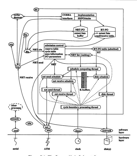
Figure 7.4: The Storage Node Software Structure
