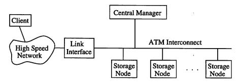
Figure 3.5: The MARS Prototype Architecture
