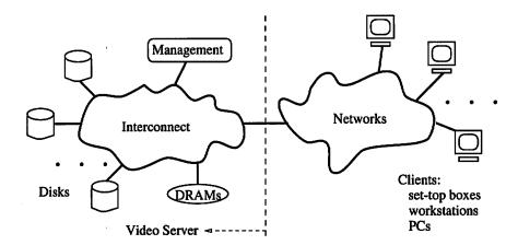
Figure 2.2: Basic Video Server System Structure
