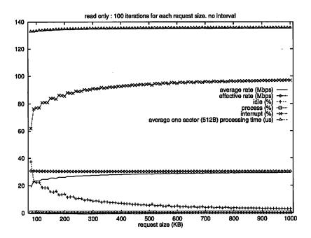
Figure 8.8: Disk Read with Increasing Request Size
