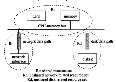
Figure 6.1: Fundamental Resources in an SS Entity
