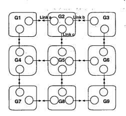
a. An array of nine switching nodes is decomposed into nine grains
