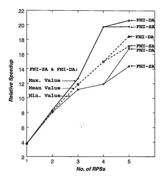
Figure 7.8: Relative Speedup obtained when simulation runs are performed by different numbers of RPSs (Scenario One: two DEC3100 clusters; each cluster has 24 workstations.)
