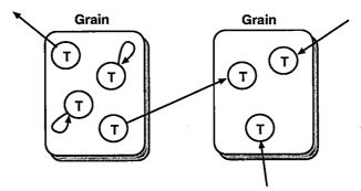
Figure 4.11: Intra-/Inter-Grain Relocation of Tasks
