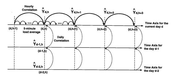
Figure 5.2: Workstation Load Forecasting
