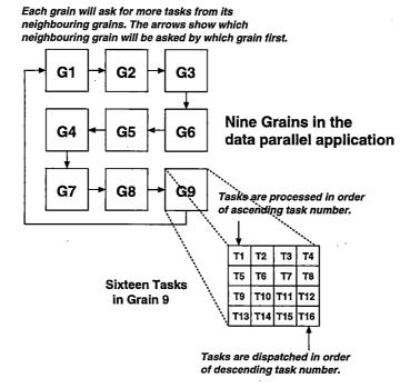
Figure 4.3: The LWD for Data-Parallel Applications
