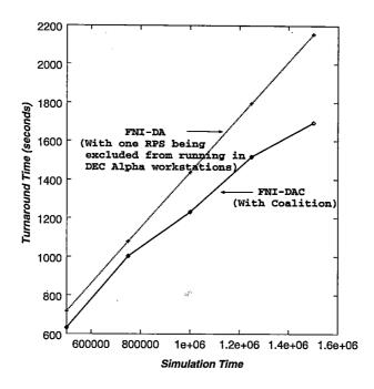
Figure 7.14: Performance of the FNI-DA and FNI-DAC policies for different simulation times (Scenario Two: two heterogeneous clusters; one has 30 DEC3100 workstations, the other has 6 DEC Alpha workstations.)
