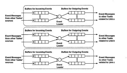
c. The Decomposed Tasks of the Switching Node (G2)
