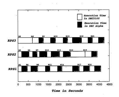
Figure 7.13: The execution time of three RPSs in DEC3100 and DEC Alpha clusters; each simulation run takes 1 million time units (Scenario Two: two heterogeneous clusters; one has 30 DEC3100 workstations, the other has 6 DEC Alpha workstations.)
