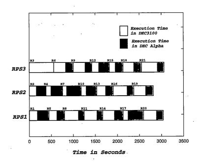
Figure 7.12: The execution time of three RPSs in DEC3100 and DEC Alpha clusters; each simulation run takes 0.75 million time units (Scenario Two: two heterogeneous clusters; one has 30 DEC3100 workstations, the other has 6 DEC Alpha workstations.)
