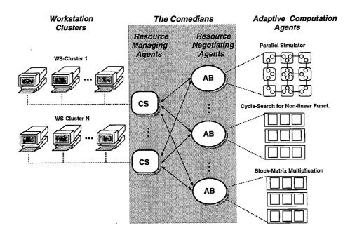
Figure 6.2: System Architecture that supports Adaptive Parallel Applications
