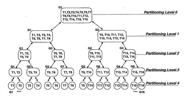
Figure 3.3: Splitting and merging of the grains (by a factor of two) of an application between different partitioning levels
