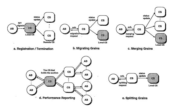
Figure 6.3: Interaction between ABs and local and remote CSs
