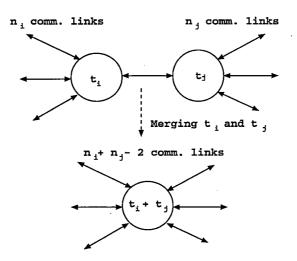
Figure A.4: Merging of two tasks
