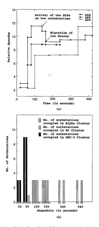
Figure 6.8: Relative speedup and snapshots of the experiments in the second scenario: there are three clusters, one has 6 DEC Alpha, the second one has 5 HP, and the third one has 30 DEC3100.
