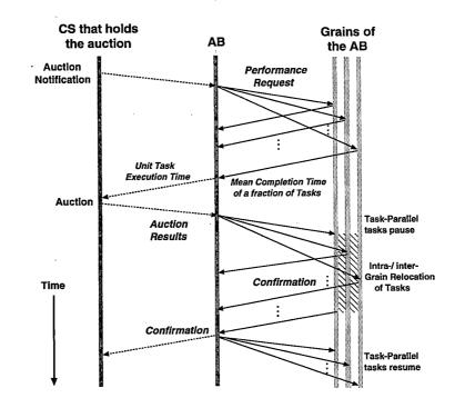
Figure 5.7: Interaction between Cluster Scheduler (CS), Application Bidder (AB), and Grains during an auction
