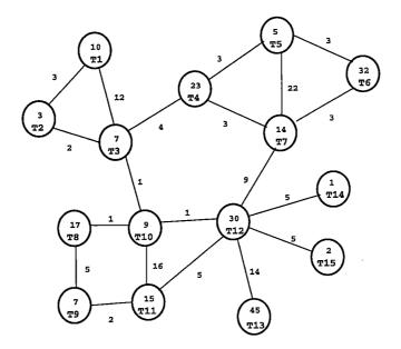
Figure A.1: The Task Graph of an Application
