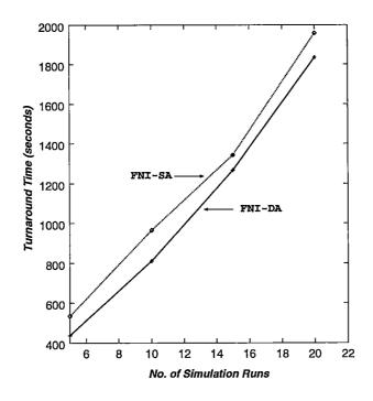
Figure 7.10: Performance of the FNI-SA and FNI-DA policies for different numbers of simulation runs (Scenario One: two DEC3100 clusters; each cluster has 24 workstations.)
