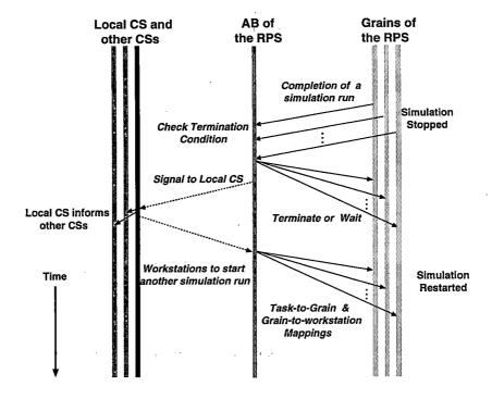
Figure 7.7: Interaction between the Cluster Schedulers (CSs), Application Bidder (AB), and Grains of an RPS during a simulation restart.
