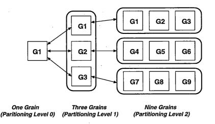
Figure 4.9: Grain Merging and Splitting for the Data-Parallel Applications
