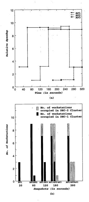
Figure 6.7: Relative speedup and snapshots of the experiments in the first scenario: there are two clusters, each has 10 DEC3100.
