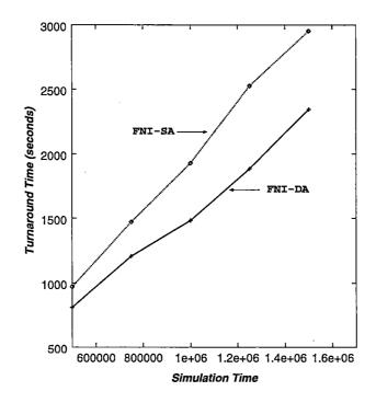
Figure 7.9: Performance of the FNI-SA and FNI-DA policies for different simulation times (Scenario One: two DEC3100 clusters; each cluster has 24 workstations.)
