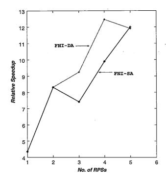
Figure 7.11: Relative Speedup of the FNI-SA and FNI-DA policies when there is one alien application running on the first cluster (Scenario One: two DEC3100 clusters; each cluster has 24 workstations.)
