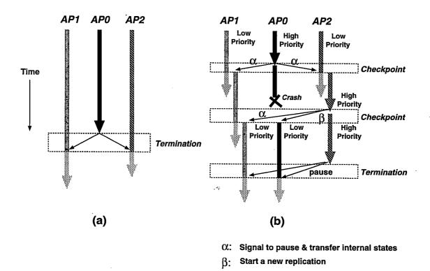
Figure 7.2: (a) Replicated Parallel Applications without Checkpoints; (b) Replicated Parallel Applications with Checkpoints
