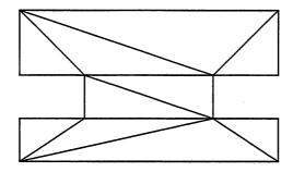
Figure 5.12: Mesh generated by removal of individual elements
