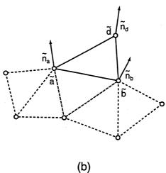
Figure 6.9: Determining the curvature of a triangle: normal vectors in world space (a) and deformed space (b)
