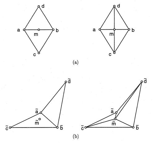
Figure 5.6: Edge splitting in undeformed (a) and deformed (b) space
