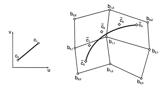
Figure 3.1: Mapping of a straight line in parameter space into world space
