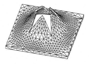
Figure 7.9: Mesh of bell-shaped tile.  $\varepsilon_{\rm max}=0.2,\,2920$  triangles
