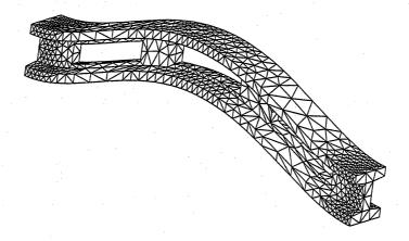
Figure 7.13: Mesh of deformed girder.  $\varepsilon_{\rm max} = 0.05,\,2668$  triangles
