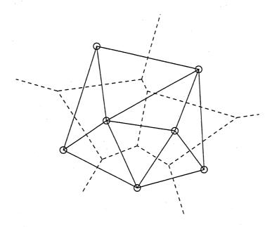
Figure 5.10: Voronoi diagram (dashed) and Delaunay triangulation
