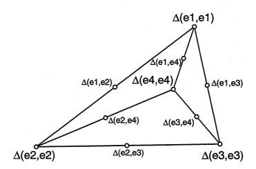
Figure 2.13: Control points of a Bézier tetrahedron
