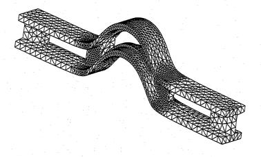
Figure 7.15: Mesh of B-spline deformed girder.  $\varepsilon_{\rm max}=0.1,\,6378$  triangles.
