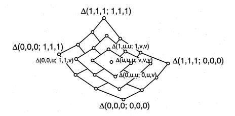
Figure 2.12: Direct evaluation of a point (u, v) on the surface of a bicubic tensor product Bézier patch over the interval  $[0, 1] \times [0, 1]$
