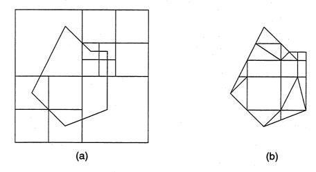
Figure 5.15: Spatial decomposition by quad tree (a) and resulting mesh before smoothing (b)
