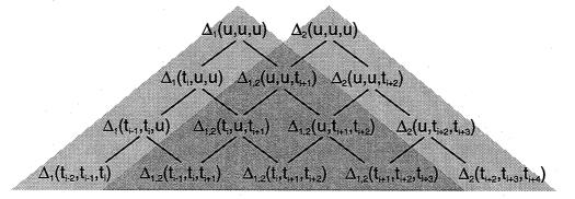
Figure 2.9: De Boor points for two adjacent cubic B-Spline segments
