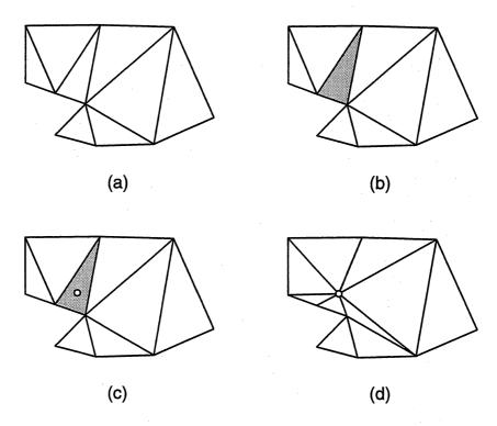
Figure 5.11: Mesh generation by selective refinement: Boundary triangulation (a), identification of a too large triangle (b), placement of new node (c), update of triangulation (d)
