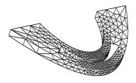
Figure 7.6: Meshed solid for  $\varepsilon_{\text{max}} = 0.1$ , 1606 triangles
