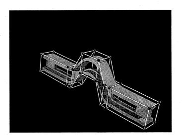
Figure A.6: Girder deformed by non-uniform B-spline,  $\varepsilon_{\rm max}=0.1$
