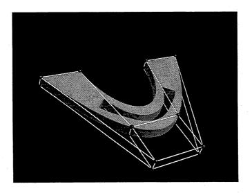
Figure A.3: Planar deformation of solid with  $\varepsilon_{\rm max}=0.1$
