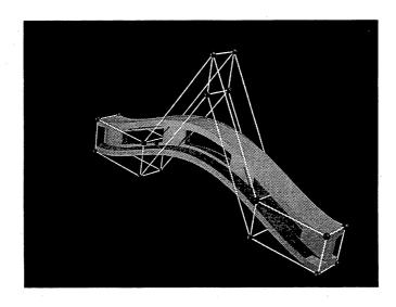
Figure A.5: Deformed girder with  $\varepsilon_{\rm max}=0.05$
