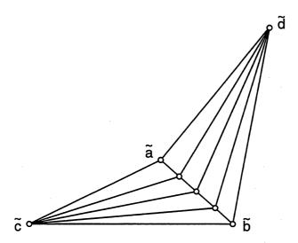
Figure 5.4: Generation of triangles of poor shape by repeated division of a triangle along the same edge
