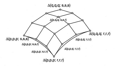
Figure 2.11: The control point net for a bicubic tensor product Bézier patch
