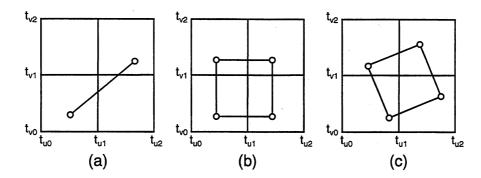
Figure 3.9: Deformation by B-spline patch: curve (a), aligned Bézier patch (b), general Bézier patch (c)
