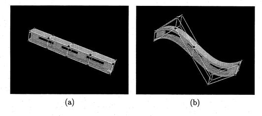
Figure 1.1: Free Form Deformation of a girder
