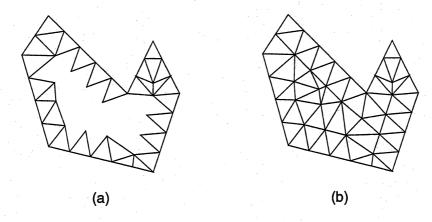
Figure 5.14: Advancing front: propagation of the front (a) and final mesh (b)
