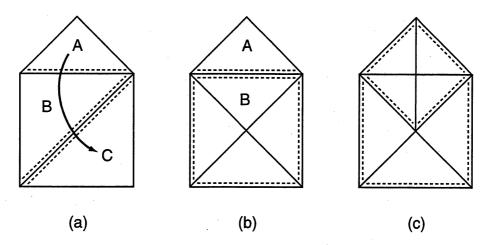
Figure 5.5: Mesh refinement with Parry's algorithm: long sides are shown as dotted lines
