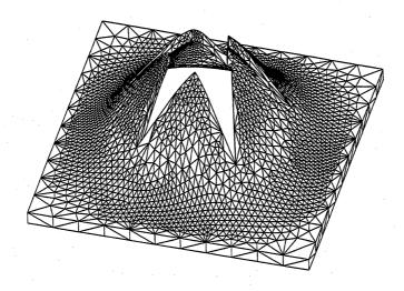
Figure 7.10: Mesh of bell-shaped tile.  $\varepsilon_{\rm max}=0.1,\,9230$  triangles
