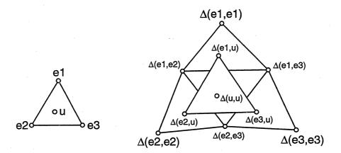
Figure 2.10: The de Casteljau algorithm for a quadratic Bézier triangle
