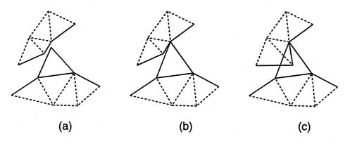
Figure 6.6: Rejection of a node: too close to existing edge (a), existing node too close to newly created edge (b), existing edge intersects new edge (c)
