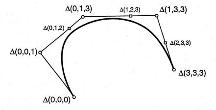
Figure 2.8: Knot insertion into a cubic B-spline curve. The original knot vector is  $\{0,0,0,1,3,3,3\}$ , we insert knot 2 and obtain the new knot vector  $\{0,0,0,1,2,3,3,3\}$
