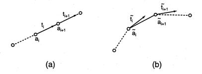
Figure 6.7: Subdivision of edge according to tangent vectors: world space (a) and deformed space (b)
