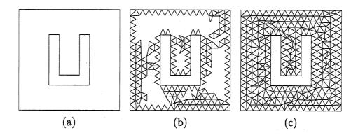
Figure 6.2: Generation of a mesh for a planar domain
