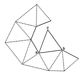
Figure 6.4: Construction of a candidate vertex **c** for a new triangle
