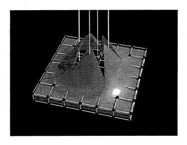
Figure A.4: Bell-shaped deformation of tile with star-shaped hole,  $\varepsilon_{\rm max}=0.2$
