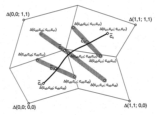
Figure 3.5: Reparametrisation of a biquadratic Bézier patch: final Bézier points
