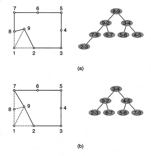
Figure 6.3: Generation of a new triangle in the domain (left) and updating the heap structure. The solid line indicates the current front.
