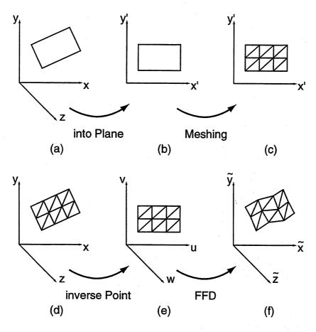
Figure 6.1: Domain in world space (a), transformation into plane (b), meshing (c), retransformation into world space (d), transformation into local solid space (e), FFD (f)
