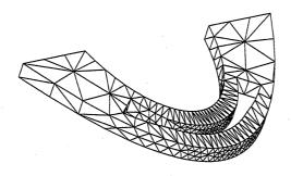
Figure 7.7: Meshed solid without planar distortion detection.  $\varepsilon_{\rm max}=0.1,$  884 triangles
