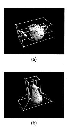
Figure 4.1: Turning the teapot into a jug: Definition of the deformation solid (a), deformation of the solid results in deformation of the enclosed teapot (b)
