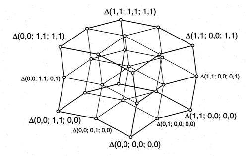
Figure 2.14: The control point net for a triquadratic tensor product Bézier Volume
