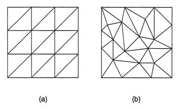
Figure 5.8: Structured (a) and unstructured (b) mesh
