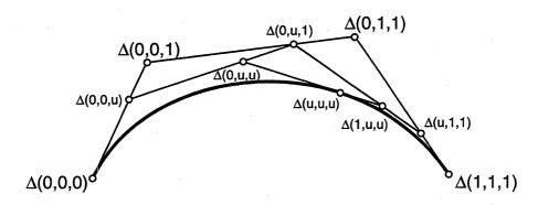
Figure 2.1: The De Casteljau algorithm for a cubic Bézier curve
