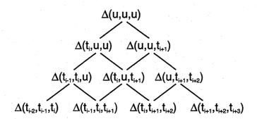
Figure 2.6: Recursive Generation of intermediate points for a cubic B-spline curve
