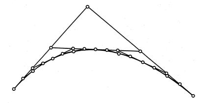
Figure 5.1: Approximation of a quadratic Bézier curve by repeated subdivision
