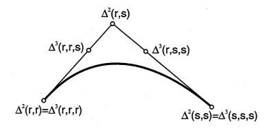
Figure 2.4: Degree elevation of a quadratic Bézier curve
