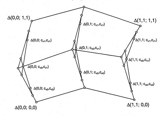
Figure 3.3: Reparametrisation of a biquadratic Bézier patch: intermediate Bézier points
