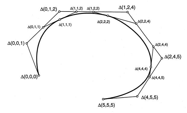
Figure 2.7: The de Boor algorithm for a cubic B-spline curve with knot vector  $\{0,0,0,1,2,4,5,5,5\}$
