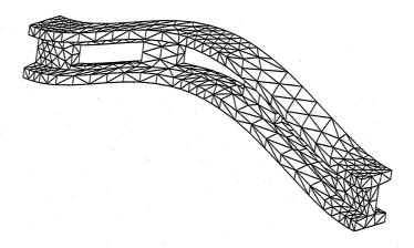
Figure 7.12: Mesh of deformed girder.  $\varepsilon_{\rm max}=0.1,\,1402$  triangles
