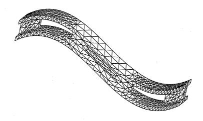
Figure 1.2: Deformed girder, 2318 triangles
