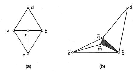
Figure 5.2: Crack caused by t-vertex
