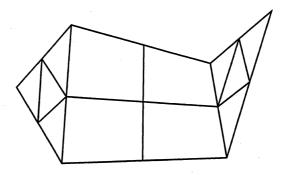
Figure 5.13: Subdomain removal and subsequent mapped meshing
