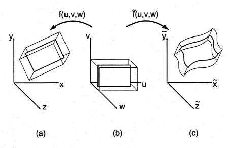
Figure 4.2: Surface in world space (x, y, z), parameter space (u, v, w) and deformed space  $(\tilde{x}, \tilde{y}, \tilde{z})$
