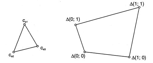
Figure 3.6: Mapping of a linear Bézier triangle onto a bilinear Bézier patch
