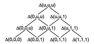
Figure 2.2: Recursive generation of intermediate points for the cubic case
