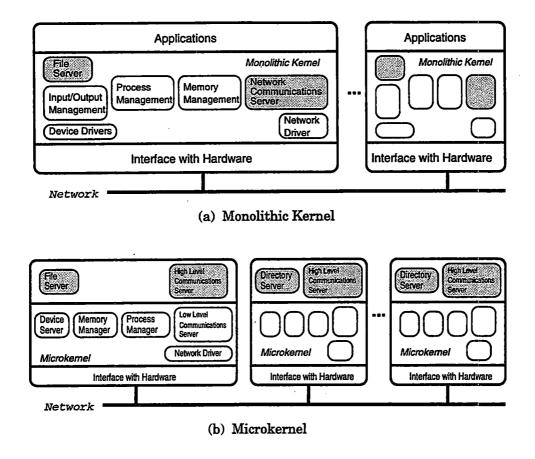
Figure 2.1: Monolithic Kernel vs. Microkernel
