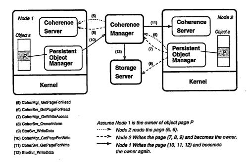
Figure 4.4: Illustration of the Centralised-Control Protocol
