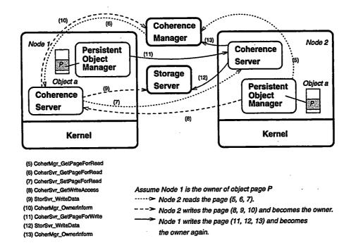
Figure 4.5: Illustration of the Distributed-Control Protocol
