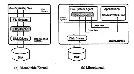
Figure 2.2: File Access in Monolithic Kernels and Microkernels
