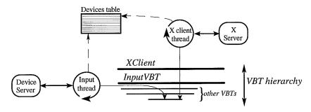
To add an input device, an application inserts an InputVBT at the top of its VBT tree and attaches a Device object to it. This can be seen in Figure 9-6: the XClient at the top provides the main window,
