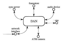
A DAN can be thought of as a small distributed system with devices, such as displays, cameras, and processors, directly connected to an ATM switch. Figure 4-2 shows a DAN with, amongst other devices, a framestore and audio device; a *synchronisation server* (see [Sreenan93]) may be used between the incoming connection and the output devices to ensure "lip-synchrony" for networked
