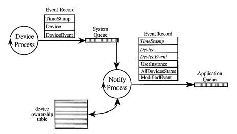
Figure 8-9 summarises the processes and queues used in input handling. When the user manipulates an input device, MMM's *device process* builds an *event record* to represent this event and fills in the time when the event occurred, the device, and the event type (mouse movement or key press, for example). The record is then placed on the system queue. The device process runs at a high priority so
