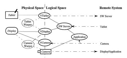
This approach allows the application and SW Server to run entirely in the DDD logical space; all the warping is managed by virtual devices so new hardware, and new *types* of hardware, can be introduced simply by connecting to different services.
