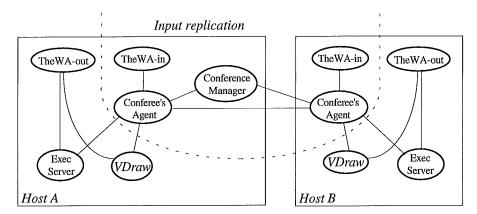
Figure 3-4. Replication of input for VDraw in TheWA window system.
