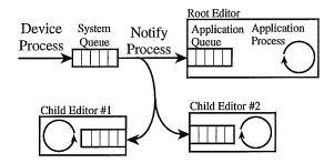
The editors are arranged in a tree; the editor at the root can have any number of child editors, each of which can have any number of children and so on (recall Figure 8-5). Each editor has an *application queue* of input events and its own lightweight *application process* (a thread) to dequeue and execute events (Figure 8-8). When an editor receives an input event, it may act on the event immediately, place it on its queue for sequenced execution, or pass it to a child editor.
