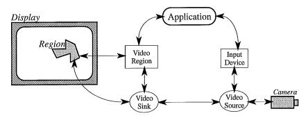
The VideoDisplay. Region establishes a link between a video sink and a display and provides access through its event handlers to the out-of-band data which is relevant to the user interface layer.
