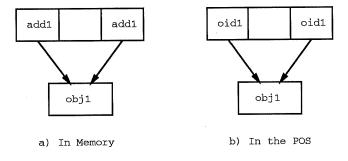
Figure 8.6: Preserving Referential Integrity in PC++
