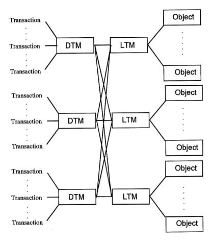
Figure 5.1: The Architecture of the Distributed Transaction System
