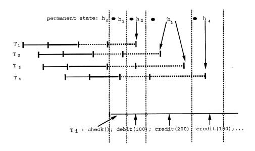
Figure 4.1: Permanent States When Executing Operations
