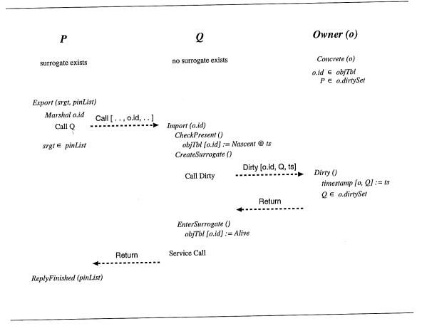
Figure 5.1: Overview of reference transmission.
