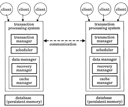
Figure 10 A distributed transaction processing system.
