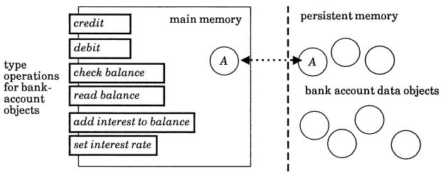
Figure 1 An example of a persistent object: a bank account object.
