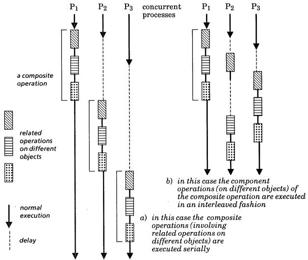
Figure 3 Execution of a composite operation by concurrent processes.
