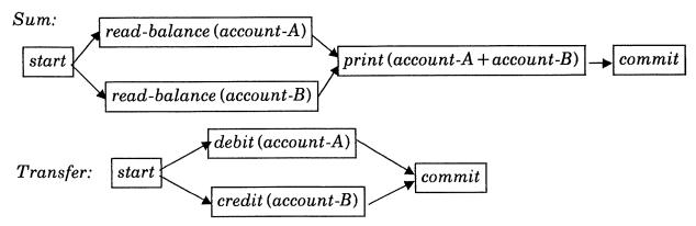
Figure 4 Graphical representation of the Sum and Transfer transactions.
