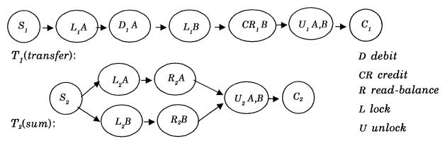
Figure 12 Two transactions including lock and unlock operations.
