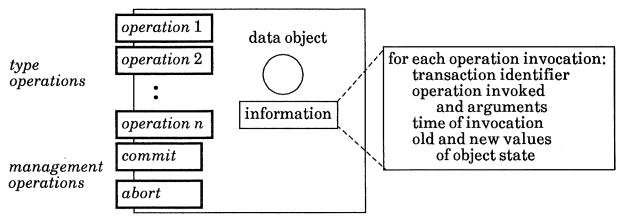
Figure 11 An object used in a transaction system.
