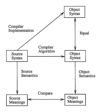
Figure 5: Combining Specification Correctness and Implementation Correctness
