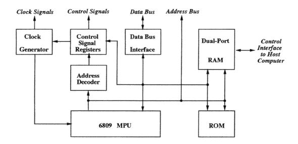
Figure 7.3: Block Diagram of NVST Controller
