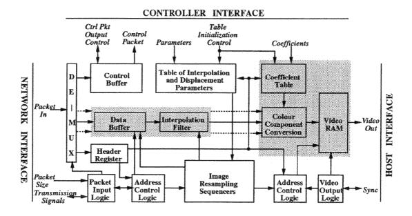
Figure 7.4: Block Diagram of NVST Receiver
