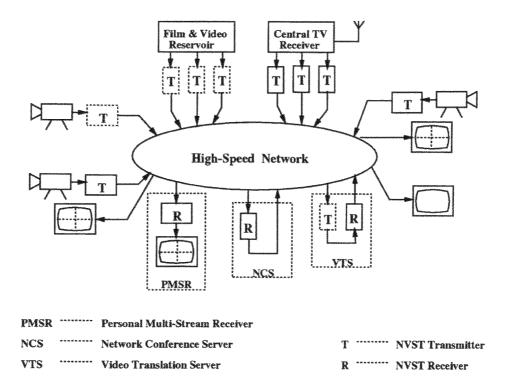
Figure 7.12: Applications of the Network Video Stream Transceiver Systems
