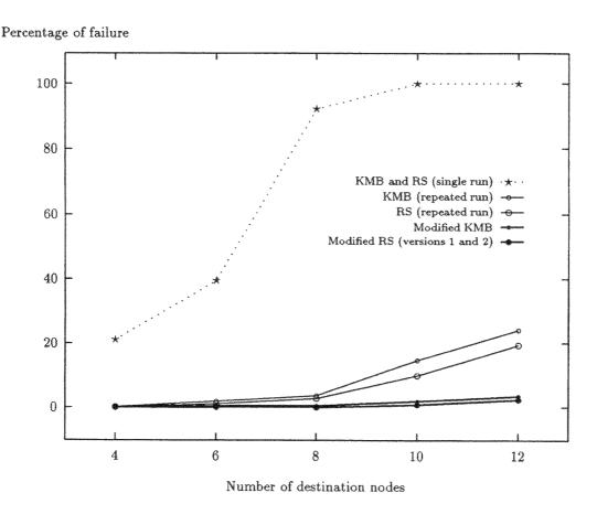
Figure 4.4: Failure Rates of the Routing Algorithms
