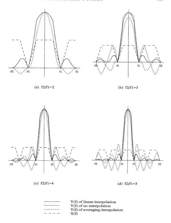
Figure 7.6: Frequency Spectra of Input and Output Streams
