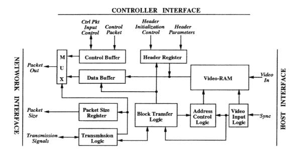
Figure 7.2: Block Diagram of NVST Transmitter
