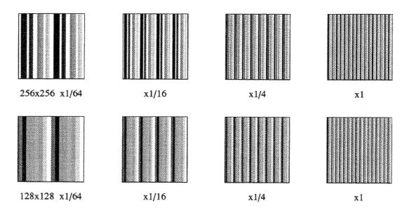
Figure 7.8: Test Pattern 2 — Grey Shading with White Stripes
