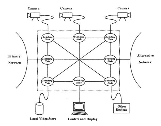
Figure 4.7: A Multimedia Switching Subsystem
