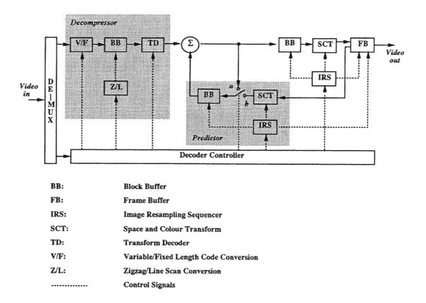
Figure 6.4: Structure of A Universal Decoder
