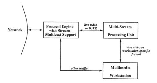
Figure 7.13: A Configuration for Multipoint Digital Video Communications
