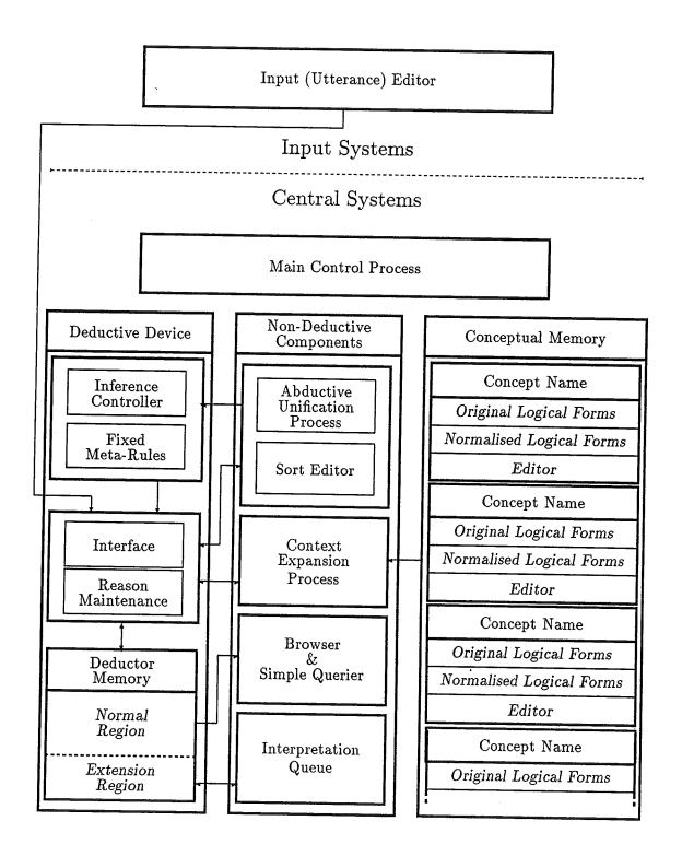
Figure 3.2: System Perspective of Crystal
