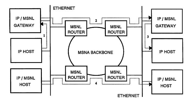
Figure 4.2: Sample IP over MSNL Configurations
