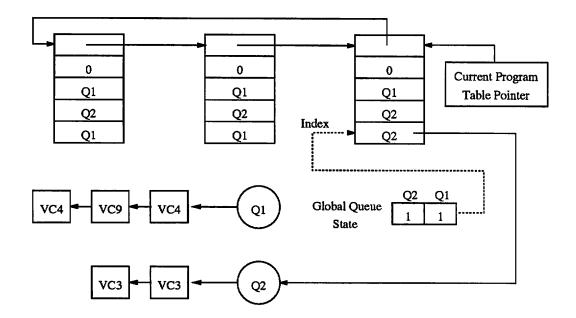
Figure 6.2: Example Two Queue Transmission Program
