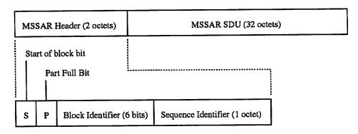
Figure 2.10: MSSAR PDU encoding
