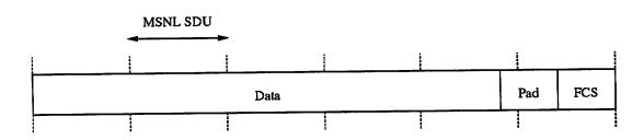
Figure 2.11: Simplified Block Assembly Protocol
