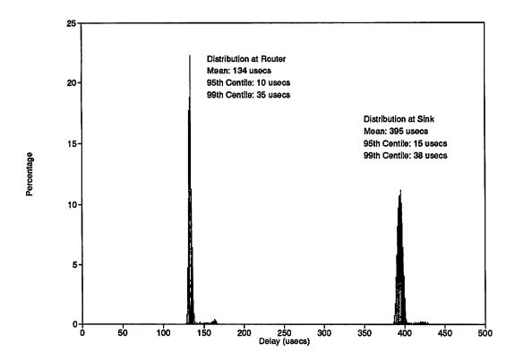
Figure 7.6: Single Cell Stream: CBN/CFR Router
