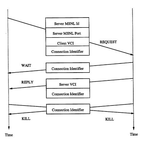
Figure 2.9: MSNL Liaison Establishment and Tear Down
