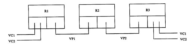
Figure 2.8: Virtual Path Call Multiplexing
