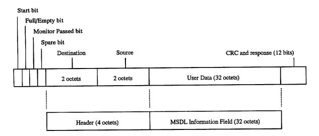
Figure 2.3: Encoding of MSDL in a CFR slot
