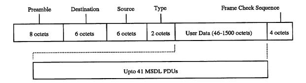
Figure 2.4: Encoding of MSDL in an Ethernet frame
