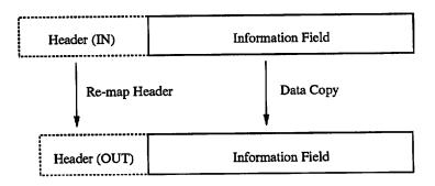
Figure 2.2: Virtual circuit gateway
