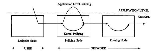
Figure 6.4: Policing Function Placement
