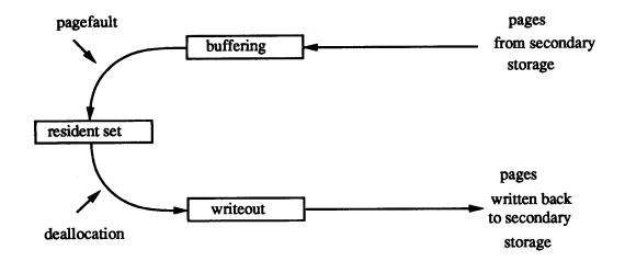
Figure 9.2: Paging for objects with highly sequential access patterns
