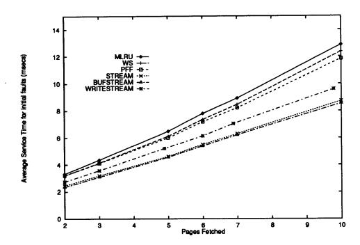
Figure 9.3: Service time for initial faults
