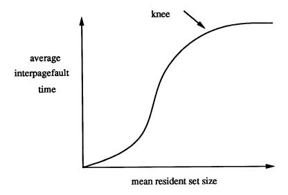
Figure 5.3: The lifetime curve
