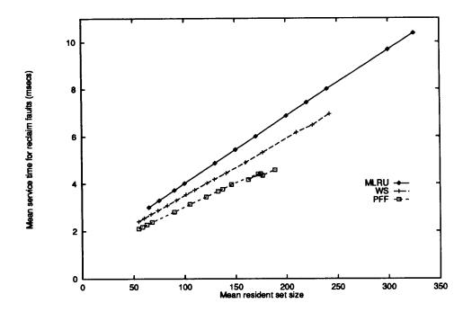
Figure 8.13: Service Time Distribution for reclaim faults for cc1
