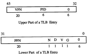
Figure 2.4: A TLB Entry for the MIPS Architecture
