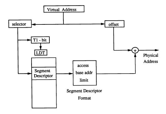
Figure 2.3: Address Resolution on the 80286
