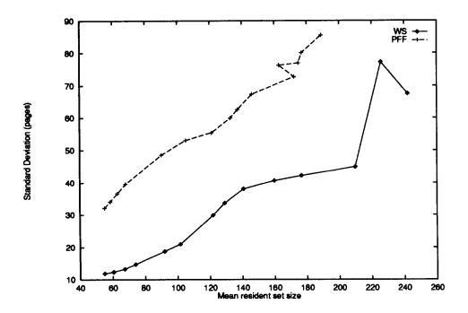
Figure 8.11: Standard Deviation vs Mean resident set size for cc1
