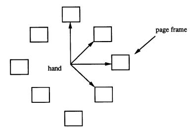
Figure 5.1: Clock Algorithm
