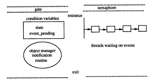
Figure 7.2: The Object Monitor
