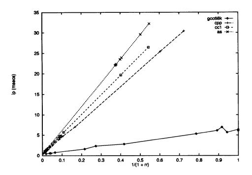
Figure 8.3: The Interpagefault Time vs 1/(1+rr) for the text segments of the Compiler Suite using the WS algorithm
