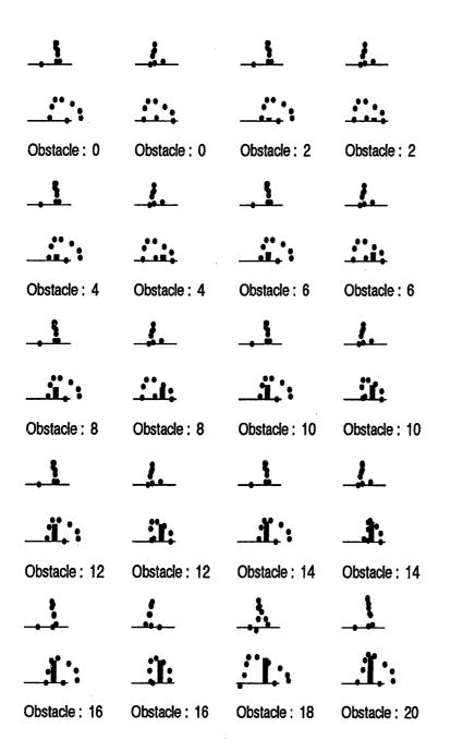
Figure 8.8: The robot tries to cross obstacles of different heights discarding the experience gained in previous attempts. It only uses the set of "strong gaits". Successful obstacle crossing gaits are *not* stored. The robot fails to lift the second leg over the obstacle at heights greater than 16.
