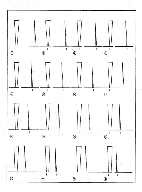
Figure 6.13: A linearised gait is executed 16 times in a row. Each picture shows the posture of the biped after the completion of a step. The regularity of the gait as well as the displacement from the right to the left are clearly visible.
