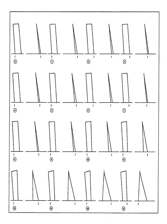
Figure 6.8: The start position selected for the fast displacement to the left. One can recognise the irregularity of the gait around the roll axis, where originally the free leg points outwards but is being pulled constantly inwards. During the last step the robot swings the free leg far too much forward around the pitch axis. However, by doing so the robot achieves a large move to the left.
