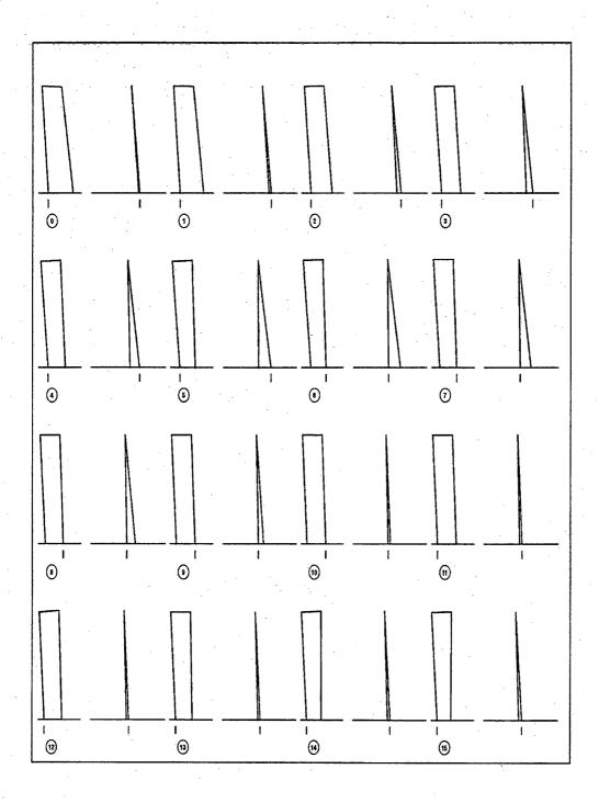
Figure 6.2: The robot walks from right to left. The small vertical line underneath the robot indicates the support leg of the robot. The robot completes a step when it changes from one foot to another. A support exchange command is carried out in positions 5, 10 and 15. Thus, the length of each step is 0.2 seconds, and the robot moves in fast short steps. On average a step is about 1.2 cm long.
