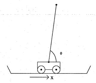
Figure 5.1: The inverted pendulum or "cart-pole" system. The cart-pole system is described using the position X and velocity X' of the cart as well as the inclination  $\theta$  of the pole and its first derivative  $\theta'$ . The system crashes when either X or  $\theta$  exceed predefined boundaries.
