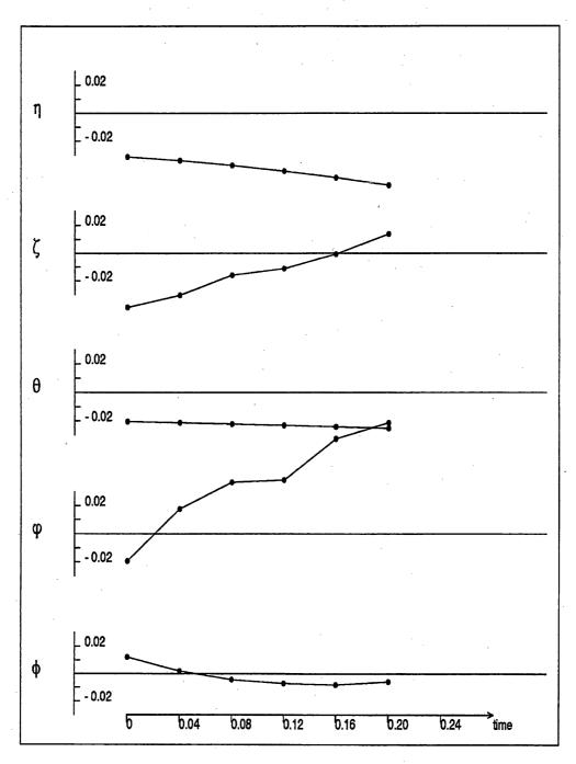
Figure 7.8: Failure of Positional Controller starting in a different start position. The controller fails after one step. Control using hip-height and displacements.
