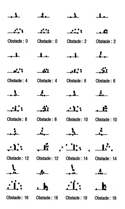
Figure 8.11: Using weak gaits and experience from previous training examples in order to cross an obstacle.
