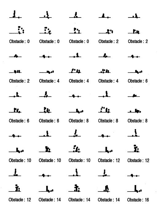
Figure 8.16: The set of strong gaits is used in order to cross a series of increasingly higher obstacles. Successful gaits are stored and used. The position described in Figure 8.15 is used as a start state. Observe that the biped fails to cross the fence at a fence height of 8mm. The biped does not succeed to lift any leg over fences which are higher than 14mm.
