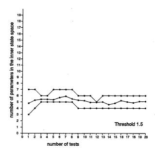
Figure 5.5: The threshold is increased to 1.5. On average only 5 parameters have an average impact on changes of the survival time above 1.5. These parameters coincide with the 5 angles describing the kinematics of the robot. The first derivatives of each angle have been filtered out.
