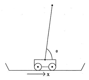
Figure 2.2: The inverted pendulum or "cart-pole" system. The cart-pole system is described using the position X and velocity X' of the cart as well as the inclination  $\theta$  of the pole and its first derivative  $\theta'$ . The system crashes when either X or  $\theta$  exceed predefined boundaries.
