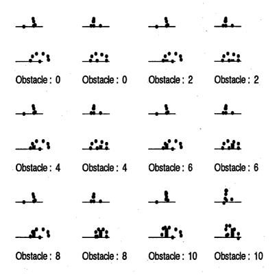
Figure 8.9: The biped tries to cross obstacles of different heights discarding the experience gained in previous attempts. It only uses the set of "weak gaits". Fences of a height of up to 10mm are crossed successfully.
