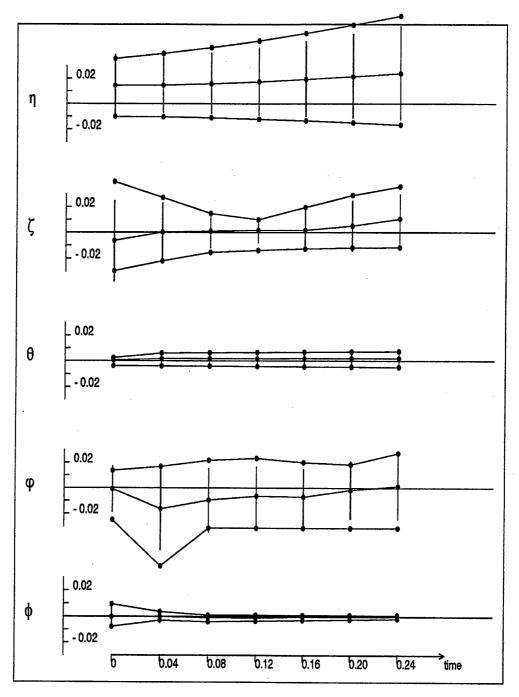
Figure 7.9: Unsuccessful use of positional controller after one search step. The robot collapsed because after 4 gait executions the free foot steps into the ground. Note that the standard deviation corresponds almost to the maximum and minimum values.
