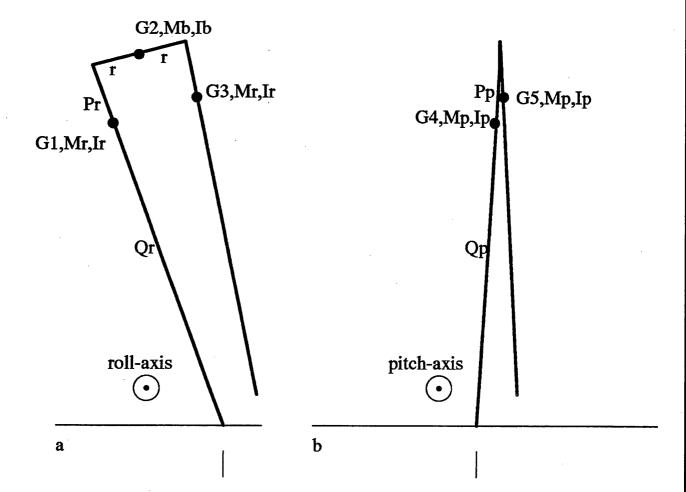
Figure 4.2: Further description of the biped model: G1,..,G5 are the centers of mass of each segment, Mr, Mb and Mp describe their respective masses, and Ir, Ib, Ip the respective moments of inertia about the centers of mass. Pr, Qr, Pp, Qp, and r describe the distance from the end of each segment to its center of mass.
