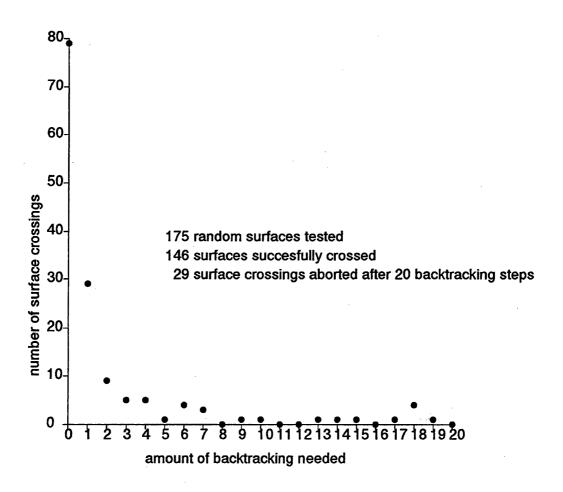
Figure 9.1: Number of backtracking needed to cross a surface with 4 randomly chosen obstacles.
