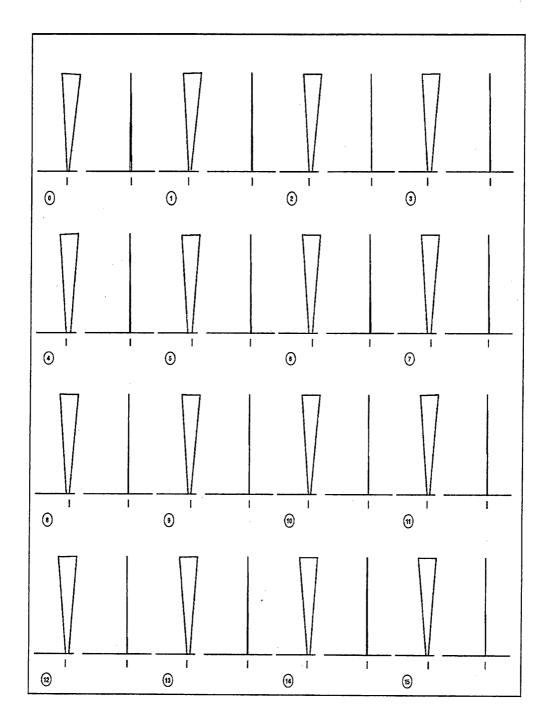
Figure 6.6: The start position selected for the most regular gait. The robot is very well balanced and there is very little movement between the frames.
