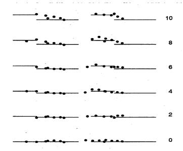
Figure 9.2: Using the qualitative equivalence heuristic to cross a step upstairs. The biped walks from the right to the left.
