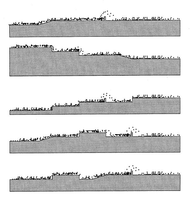
Figure 10.4: The robot crosses a sequence of random obstacles. The robot walks from the right to the left. Small black dots indicate the position of the free foot.
