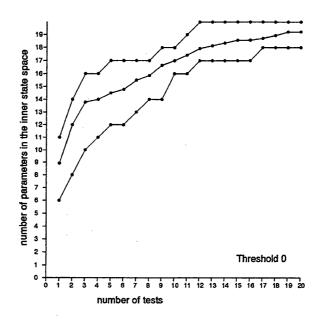
Figure 5.2: Analysis of the State Space Hierarchy,  $\theta$ =0. Any effect on survival time (average changes greater than threshold 0) were recorded. On average 19 parameters were identified which had an influence on the survival time of the robot. These parameters are the kinematic and dynamic parameters of the robot as well as the relevant parameters of the various obstacles.
