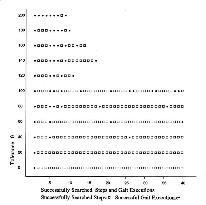
Figure 6.15: Interleaving search and gait execution. Boxes indicate search, circles indicate gait execution. The threshold (of the evaluation function) for search was increased for each trial (vertical axis). The horizontal axis indicates the time until failure. A test terminated successfully after 40 steps or gait executions.
