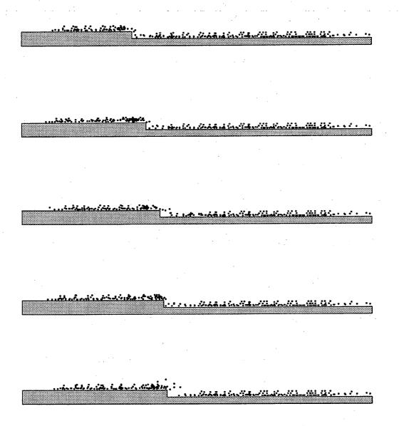
Figure 9.6: Using the virtual evaluation functions to cross a step upstairs. Each diagram represents one walk, with the position of the free foot plotted every 0.04 seconds. The biped walks from the right to the left. The location of the steps was chosen in such a way that the biped would encounter the obstacle during different moments of its stride.
