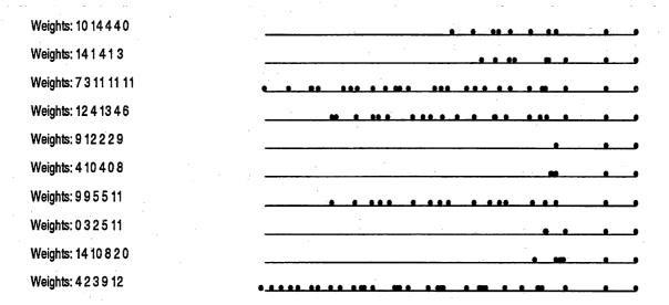
Figure 6.4: The performance of different inner state space weightings. Random weights were chosen and the robot moves from right to left. The robot is successful if it reaches the left end of the line. The weights are (from left to right) the weightings of  $\eta$ ,  $\zeta$ ,  $\theta$ ,  $\psi$ , and  $\phi$  respectively. Two inner state space weightings were successful.
