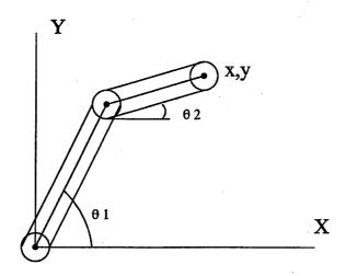
Figure 2.1: A two link manipulator
