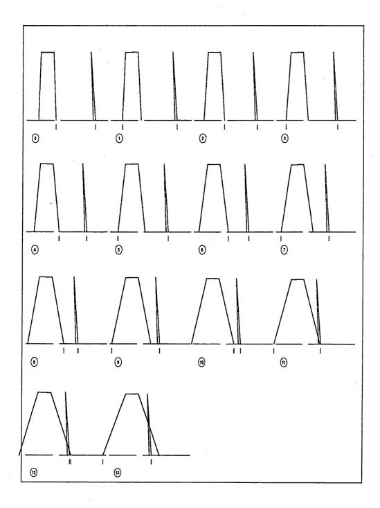
Figure 6.14: Linearised gait fails after 36 steps. Each picture shows the posture of the biped after the completion of a step. In this figure, the last 14 steps of the robot are depicted. Failure occurs because the legs of the robot are spread too far around the roll axis. The view of the pitch axis has been shifted to the right in comparison to Figure 6.13 in order to fit the two views (roll and pitch axis) into the same limited space.
