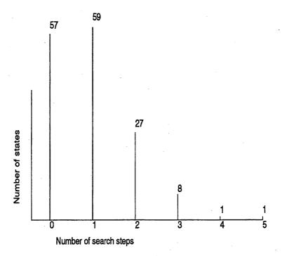
Figure 7.11: Successful use of positional control after n search steps. The diagram on the top shows the cumulative number of states which could be controlled after n steps. The lower diagram shows how many states could be controlled after n search steps, but not after n-1 search steps.
