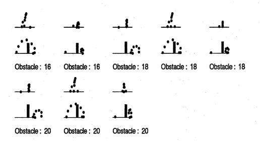
Figure 8.14: The continuation of Figure 8.13. Only one foot can be lifted over the obstacle.
