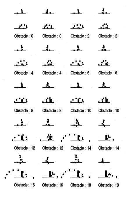
Figure 8.12: The robot crossing the obstacle, with the start position 5 units closer to the obstacle. Each successful training example is recorded, and originally the set of "weak" gaits was used. The behaviour is good for heights of up to 12 units but then deteriorates drastically: the second leg is actually moved away from the obstacle.
