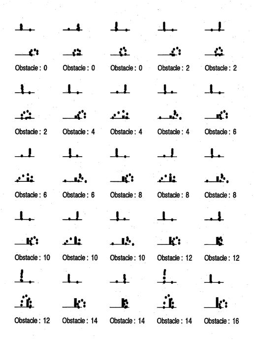
Figure 8.17: The set of weak gaits is used in order to cross a series of increasingly higher obstacles. Again the position described in Figure 8.15 is used as a start state. The obstacle crossing performance is very poor.
