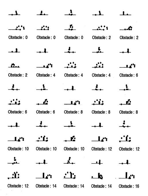
Figure 8.13: The robot crossing the obstacle, with the start position 5 units further away from the obstacle. Each successful training example is recorded, and originally the set of "weak" gaits was used. This time 3 consecutive steps are recorded. The robot fails to cross obstacles higher than 4mm.
