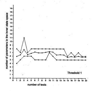
Figure 5.4: The threshold is increased to 1. About 6 parameters remain above the threshold, some first derivatives are already filtered out. The remaining parameters are the kinematic parameters of the robot and the velocity of the free leg around the pitch axis.
