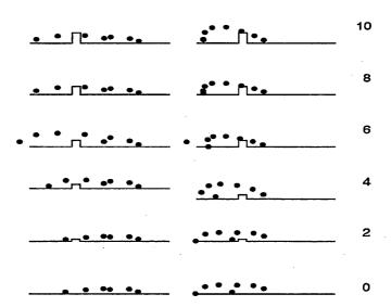
Figure 9.8: Using the qualitative equivalence heuristic to cross a fence. The height of the fence is written to the right of each plot.
