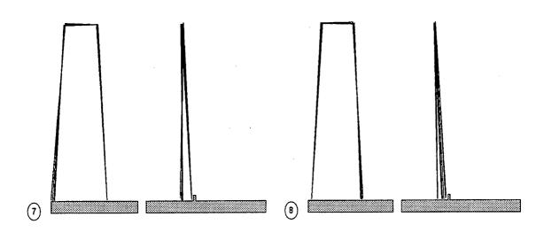
Figure 10.2: The robot lifts the second leg over the wall and resumes a posture leaning towards the left.
