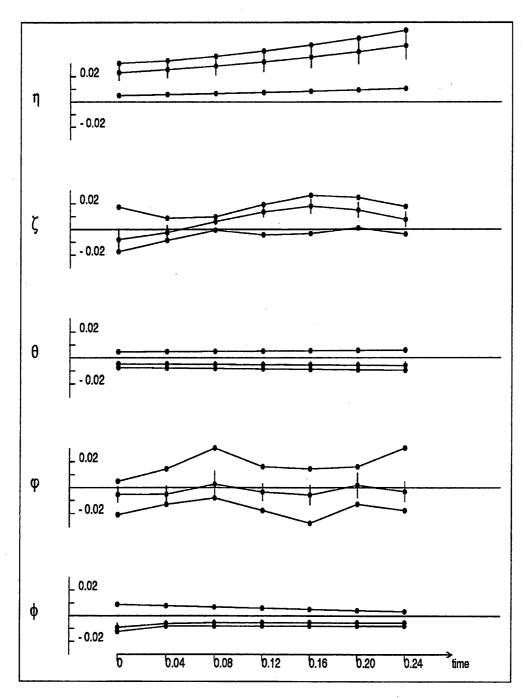
Figure 7.4: Successful use of inertial controller after two search steps. The standard deviation values decrease in comparison to Figure 7.3, indicating a more regular behaviour.
