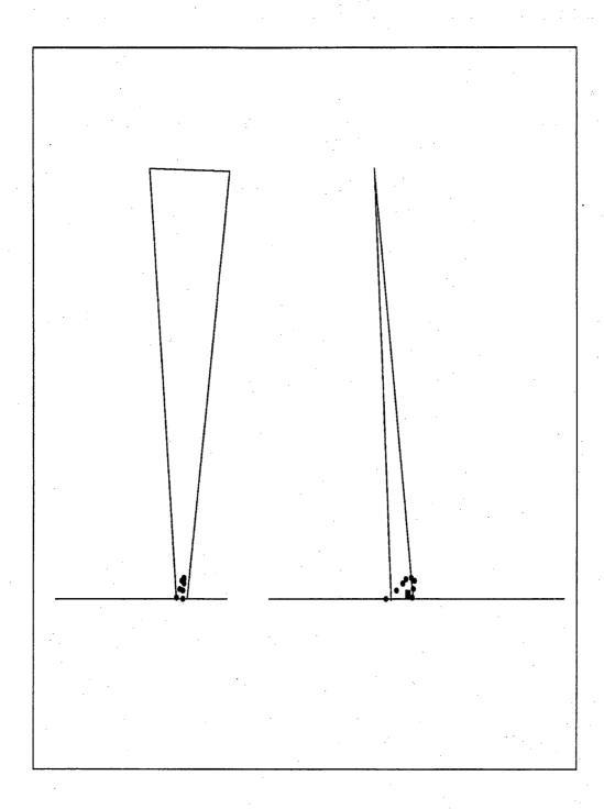
Figure 8.7: The second step of the biped over the fence. The gait modifications provide a gait which first pulls away the free leg from the obstacle and then lifts it to the other side.
