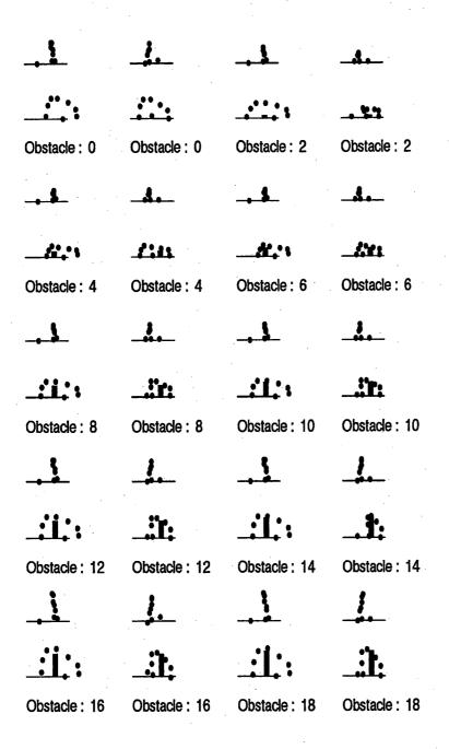
Figure 8.10: Using strong gaits and accumulating experience during the trial. The robot succeeds in crossing a 18mm high fence but fails for any higher fences. Without training the robot failed at fences higher than 16mm.
