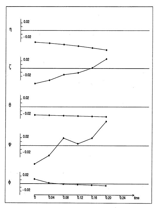
Figure 7.2: Failure of Controller due to overshoot. The biped starts in a position different from the desired start position. The biped executes only one step and then fails.
