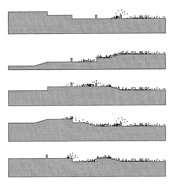
Figure 10.8: Sample of obstacle combinations which the robot was originally unable to cross
