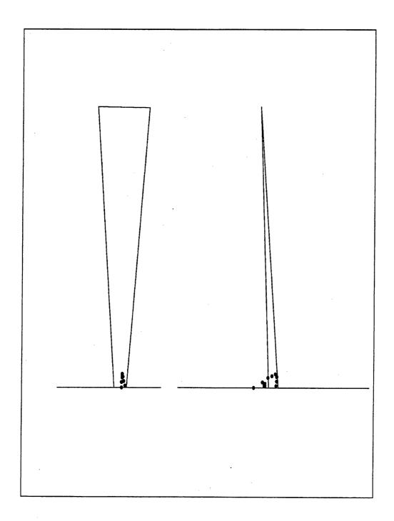
Figure 8.6: The biped crosses a small fence. The gait has been found by applying various successive gait modifications. Small black dots indicate the position of the free foot during the gait execution.
