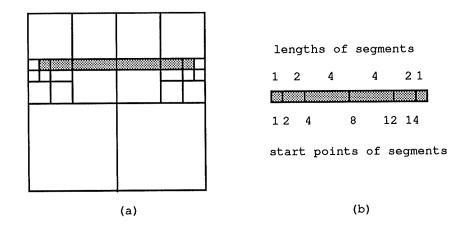
Figure 3.3: Generating a RunList from a ray: (a) a ray in a 2D region of quadtree subdivision, (b) the same ray is split into maximal segments.
