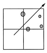
Figure 5.9: A problem of octree space subdivisions: a ray missing all objects in an octant.
