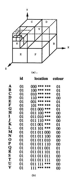
Figure 6.2: An object stored as a CAM octree for ordered retrieval: (a) the octree decomposition of the object and (b) its CAM contents
