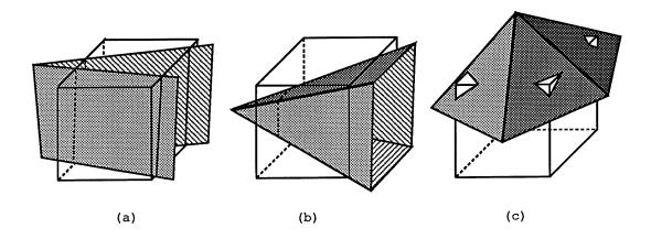
Figure 2.5: Additional leaf types for an extended vector octree: (a) an edge' cell, (b) a vertex' cell, and (c) a vertex" cell
