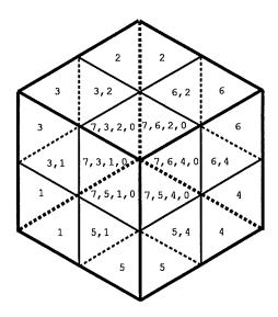
Figure 2.13: A corner view of an octree space
