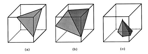
Figure 2.3: Leaf types of a vector octree: (a) a face cell, (b) an edge cell, and (c) a vertex cell
