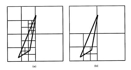
Figure 2.4: A 2D illustration of a problem with vector octrees: (a) a black hole exists when the object is in a bad position; (b) the problem can be solved by introducing more node types.
