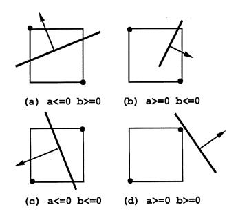
Figure 4.4: Testing two vertices to determine whether a square is inside/outside/intersecting to an arbitrary line.
