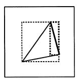
Figure 4.5: Bounding boxes for an object (the light dotted lines) and a polygon face (the heavy dotted lines)
