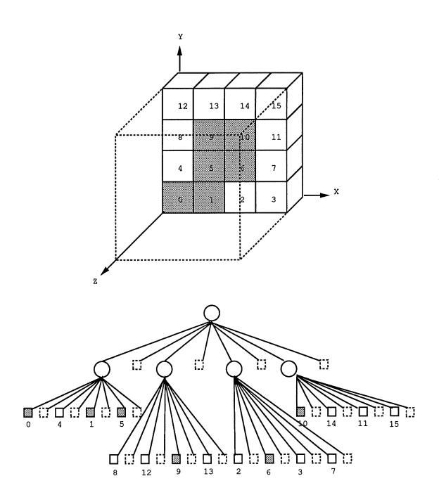
Figure 2.11: An octree for one slice of a digital image
