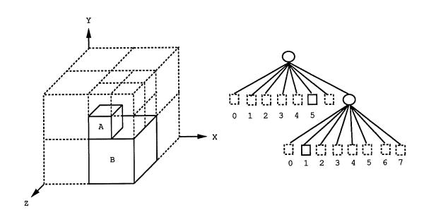
Figure 2.2: A sample object and the corresponding octree
