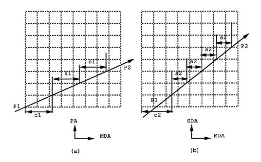
Figure 5.5: The parameters for calculating adaptive 3D-DDA: the increments (s1, s2) and the initial control terms (c1, c2)
