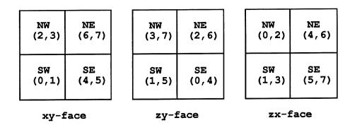
Figure 2.14: The quadrant numbers and the corresponding pseudo octree labels
