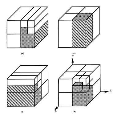
Figure 4.1: The three silhouette views ((a)(b)(c)) of an object are stored as groups of sweep volumes in the CAM, and the octree of the object (d) is obtained by intersecting these volumes.
