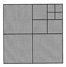
Figure 2.9: A 2D representation of nodes of a non-minimal octree
