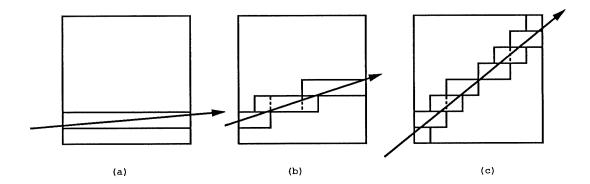
Figure 5.4: Two dimensional illustrations of adaptive 3D-DDA for rays of different orientations: (a) the best situation where the ray is nearly parallel to one axis (for instance the horizontal axis); (b) general situation; (c) the worst case where the ray enters from one corner of the world space and leaves at the opposite corner.
