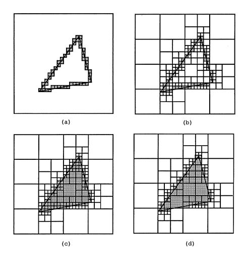
Figure 4.7: The mixed bottom-up and top-down octree construction algorithm: (a) bottom-up phase inserting boundary voxels into the CAM octree; (b) top-down phase recovering the non-boundary octants; (c) the octree after connectivity component labelling which separates internal and external octants and (d) condensing to get the minimal tree.
