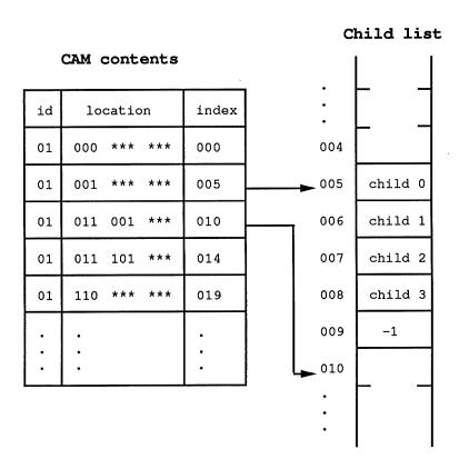
Figure 5.2: Indexing objects in a CAM octree: CAM contents and the child list.
