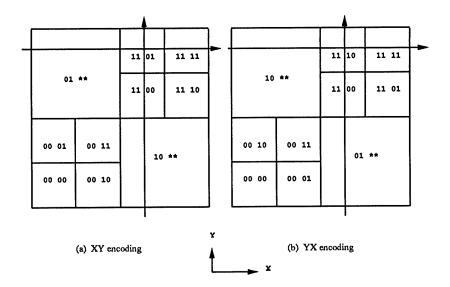
Figure 6.4: The coding scheme does not affect the order of a raster scan along any of the three axes.
