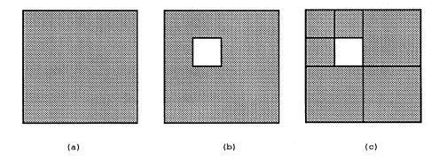
Figure 4.3: A node in (a) is split into several subnodes in (c) after inserting a small white node into a larger black node shown in (b).
