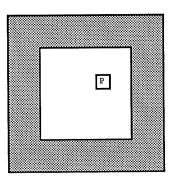
Figure 2.15: The problem of interior/exterior octant classifications for an object with a hole. The probing cell is interior to the external faces and exterior to the internal faces of the object.
