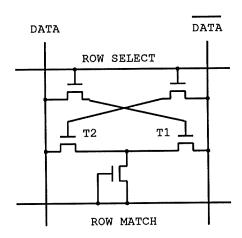
Figure 3.1: Wade and Sodini's dynamic CAM cell (courtesy of Richard Williams).
