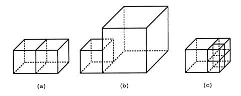
Figure 2.8: Neighbours of an octant: (a) equal, (b) larger, (c) smaller in size
