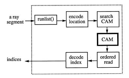
Figure 6.5: Pipelining the process of searching a CAM octree for octants intersecting with a ray.
