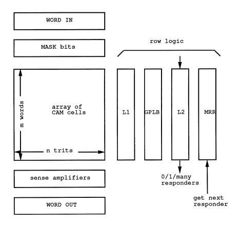
GPLB = General Purpose Logic Block MRR = Multiple Response Resolver L1, L2 = 1 bit latches
