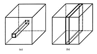
Figure 6.1: Examples of enquiry spaces: (a) a scan line, (b) a slice
