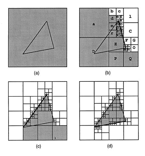
Figure 4.2: A 2D illustration of the stages of the multiple-pass top-down octree construction algorithm using CAM.
