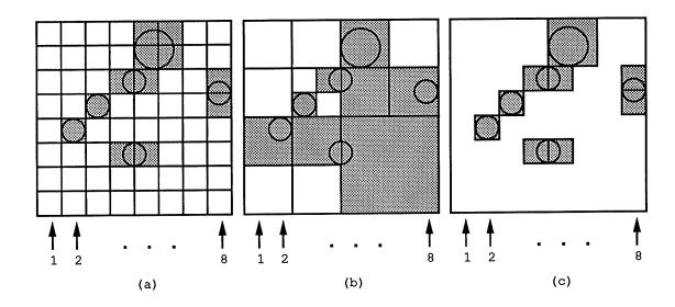
Figure 5.1: Comparison of different space subdivision schemes: (a) uniform subdivision; (b) octree subdivision; (c) proposed scheme
