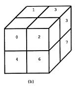
Figure 2.6: Oliver's ordinal numbers of octants for two treecode algorithms: (a) display a plane section which is parallel to the front face of the image space; (b) display an orthographic projection of an octree in a front-to-back manner.
