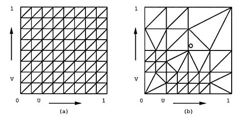
Figure 5.10: Two surface tessellation techniques: the parameter space is tessellated into triangles with (a) a uniform subdivision, (b) a restricted adaptive subdivision.
