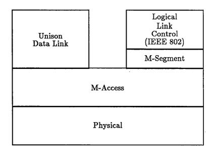
Figure 10.1: Lower Layer Protocol Architectures for the CFR
