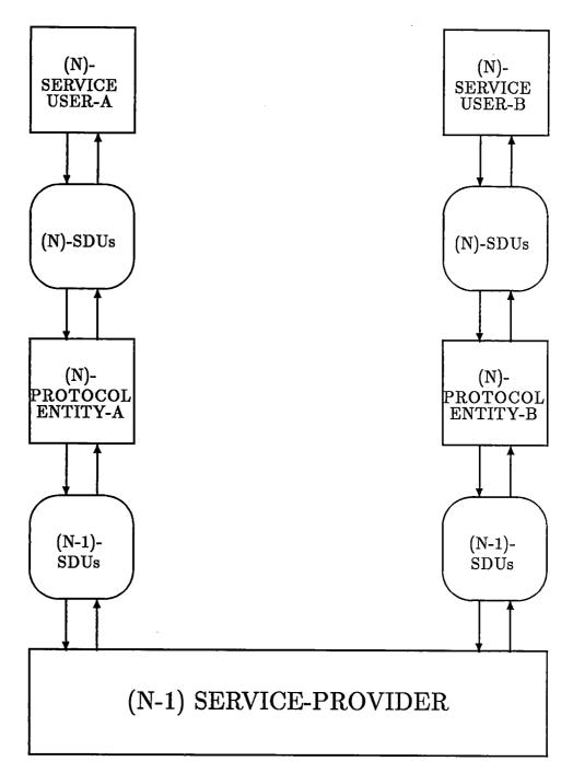
Figure 2.5: Environment for the Specification of the (N)-Protocol Entities
