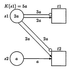
Figure 6.21: Two Inhibitors for Place S1: No concurrency
