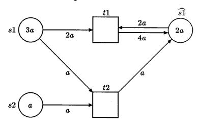
Figure 6.12: CP-net equivalent: T(P2)
