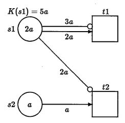
Figure 6.18: Two Inhibitors for Place S1
