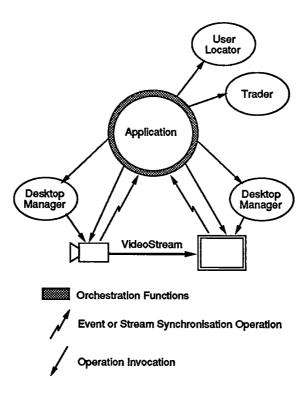
Figure 6.10: Orchestration Interaction Diagram
