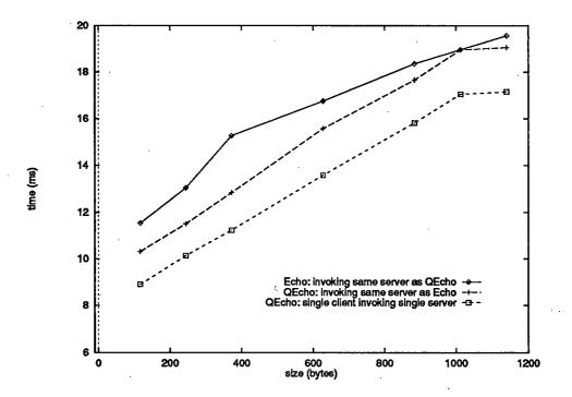
Figure 9.7: QoS Performance Using Two Clients
