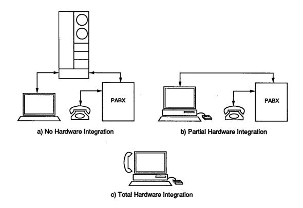
Figure 2.2: Degrees of Hardware Integration
