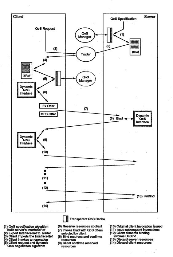
Figure 7.10: Stages In End-to-End QoS Negotiation
