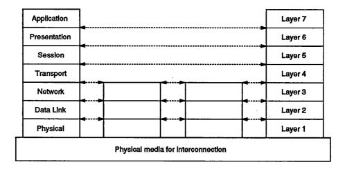
Figure 2.4: The OSI Reference Model
