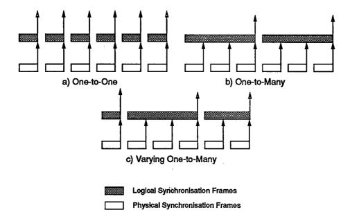
Figure 5.4: Logical to Physical Synchronisation Frame Mappings
