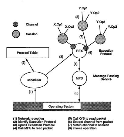
Figure 7.3: Network Reception in The Testbench
