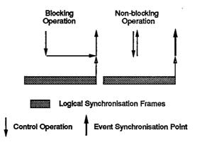
Figure 5.5: Blocking and Non-blocking Control Operations
