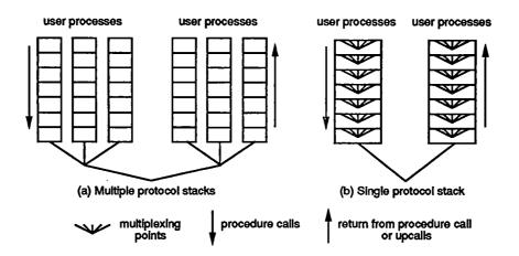
Figure 4.3: Multiple Versus Single Protocol Stacks
