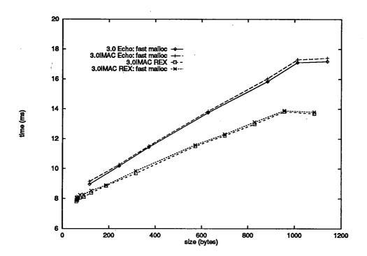
Figure 9.3: RPC Performance Using Fast Malloc
