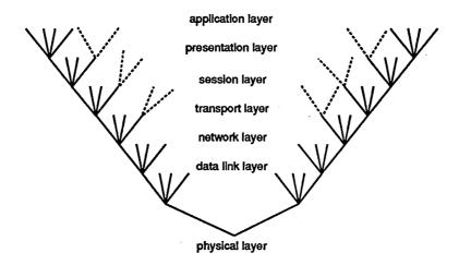
Figure 4.2: OSI Multiplexing
