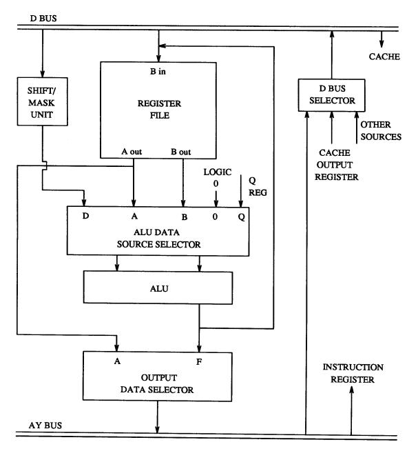
Figure 8.4: A simplified version of the AM2901C block diagram
