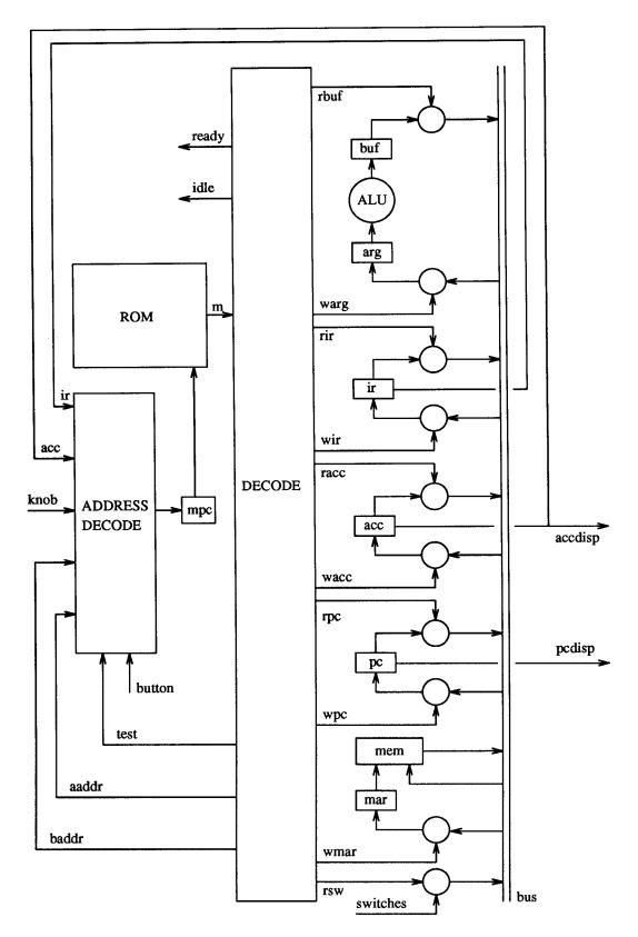
Figure 7.2: The block diagram for an implementation of Gordon's computer
