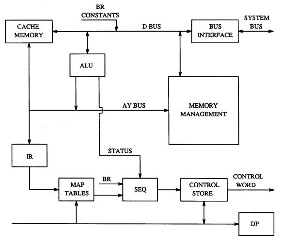
Figure 8.1: The Orion Central Processing Unit
