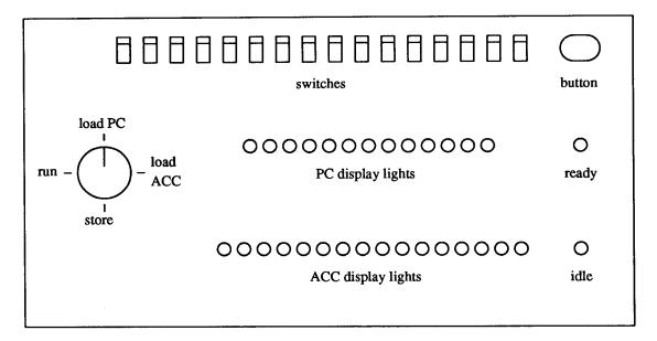
Figure 7.1: The front panel of Gordon's computer
