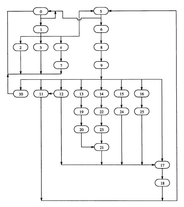
Figure 7.4: The state diagram for Gordon's computer
