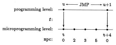
Figure 5.2: JMP Instruction Cycle Timing.
