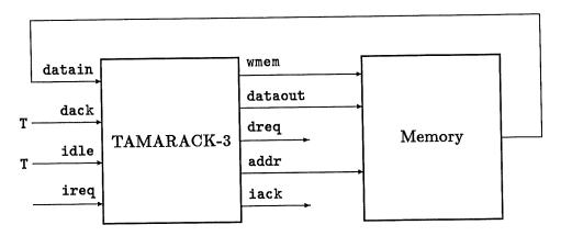
Figure 3.1: Fully Synchronous Operation.
