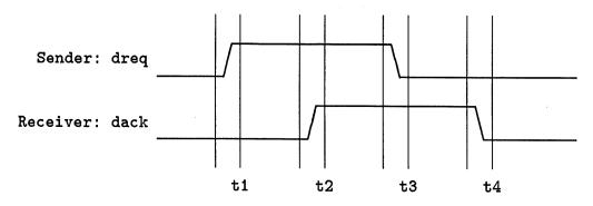
Figure 6.1: Four-Phase Handshaking Timing Diagram.
