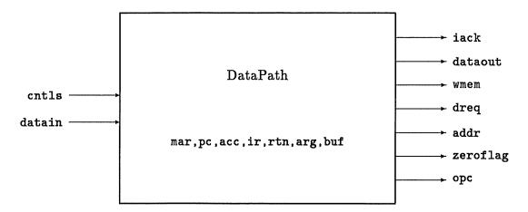
Figure 4.1: External View of the Datapath Specification
