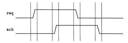
Figure 1.1: Simplified Handshaking Timing Diagram
