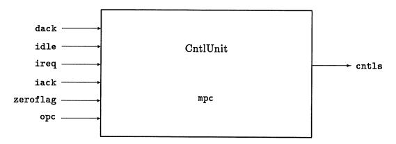
Figure 4.2: External View of the Control Unit Specification
