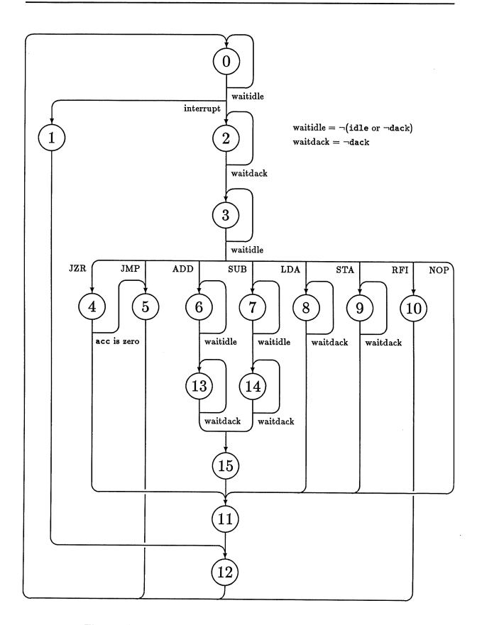
Figure 3.7: Control Unit Finite-State Machine Flow Diagram.
