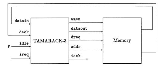
Figure 3.3: Fully Asynchronous Operation.
