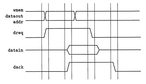
Figure 3.2: Synchronizing Data Transfer with Handshaking Signals.
