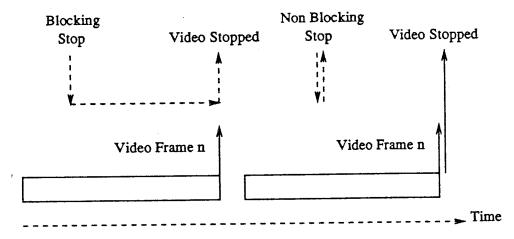
Figure 2. Blocking and Non-Blocking Control Operations
