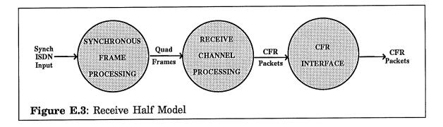
Estimates of the unpacking delay can be derived from the observation that the mapper requires a complete quad frame interval to unpack a fully populated frame.
