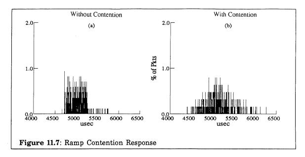
Figure 11.7(b) is an example of ramp response in the presence of periodic contention loads.<sup>1</sup> Although the overall traffic in this experiment was not sufficient to induce queueing within the ramps, the jitter spectrum has been attenuated by the batching of packet arrivals at the receive half CFR interface.
