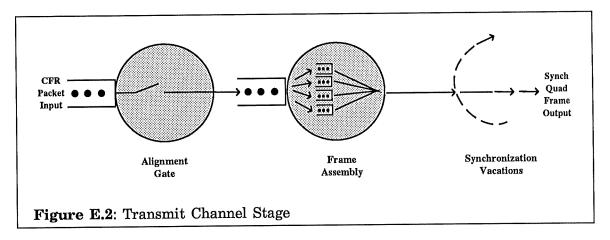
components and a single quad frame is assembled during each 500 usec cycle. In the absence of other traffic, the segments of an arriving packet are spread across some integral number of quad frames, q, determined by the number of timeslots allocated to the channel. For example, packets arriving at a single timeslot channel (q=10) will be subject to a basic delay of 5000 usec whilst packets arriving at channels of 10 or more timeslots (q=1) will be processed in a single cycle.
