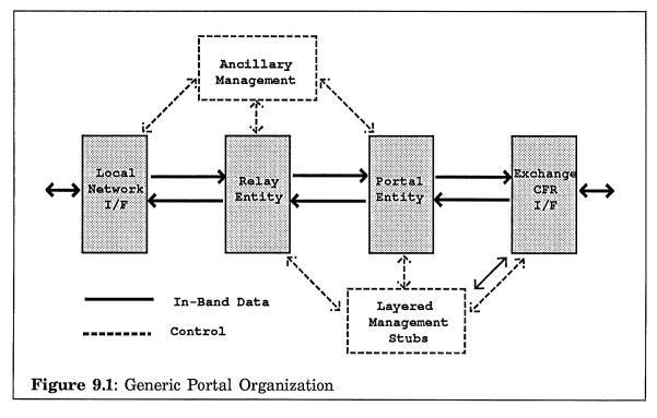
of a generic portal in which the local and exchange interfaces support the lower level gateway functions, whilst the relay, portal, and management components support the upper level functions.
