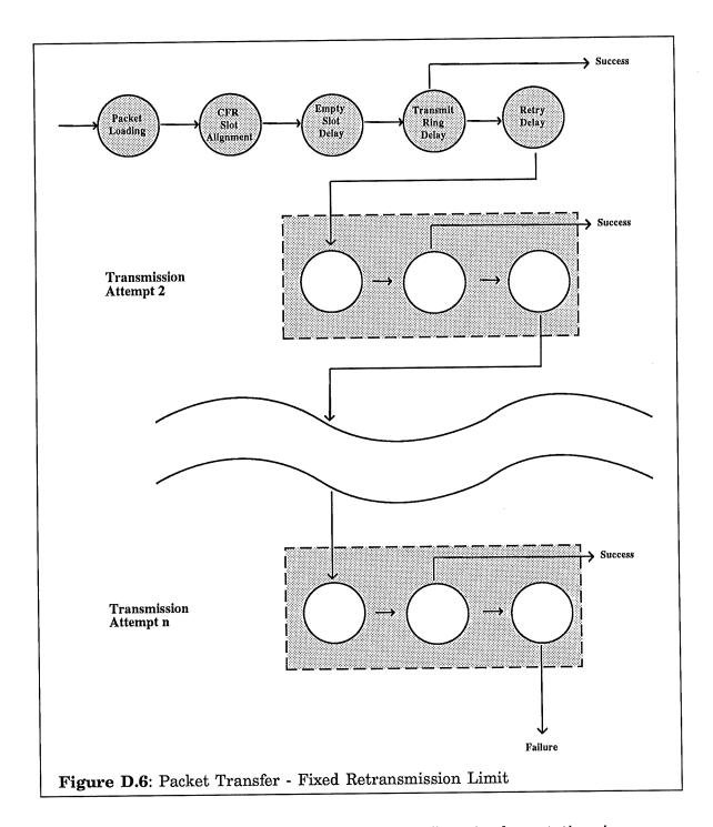
via the retry delay centre. In practice, the CFR implementation imposes a maximum limit on the number of transmission attempts and the packet transfer is aborted if this limit is exceeded. This arrangement can be modelled through replication of the appropriate delay centres as illustrated in Figure D.6.
