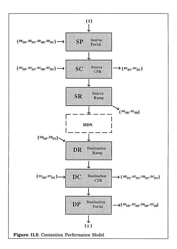
deterministic or erlangian distributions.<sup>1</sup> For modelling purposes these streams have been multiplexed together at portal, ramp, and CFR components that are external to the particular path, and whose service characteristics are unknown.
