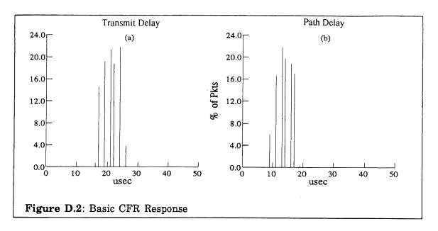
residence times were observed.¹ Given the limited accuracy of the apparatus, the transmit timer's delay range of 16 to 26 usec is consistent with the model's 15.8 usec delay component and 8.2 usec jitter component. The average of the transmit delay measurements is 21 usec versus an expected average delay of 19.9 usec.
