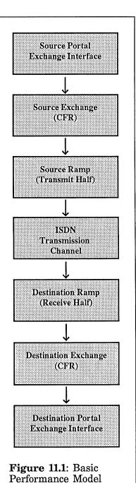
the service access points of the SI-service. The remaining portal components have been excluded from the modelling process as they are outside the scope of the SI-service and their performance is dependent on the type of client network supported.
