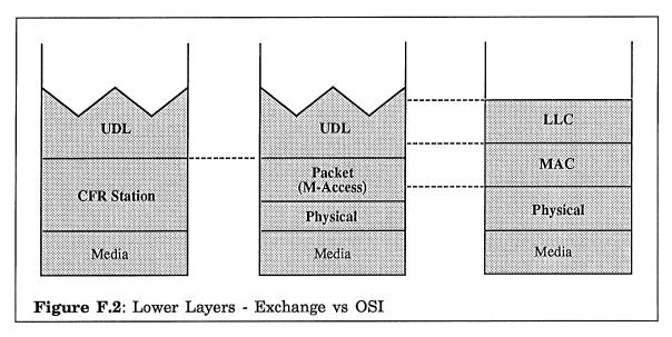
used to implement this service.<sup>1</sup> The packet layer supports the exchange of CFR packets over physical layer services and various encoding, multiplexing and switching techniques can be used within this layer. Peer ramps, operating within the packet layer, implement relaying in order to support the end-to-end exchange of symbols between packet layer uses.
