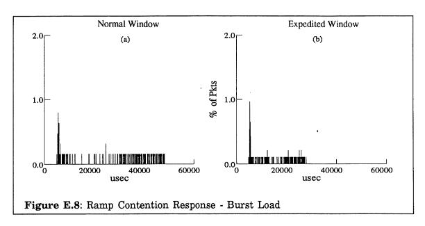
The ramp's expedited transfer function can be used to insulate jitter-sensitive traffic from the transient effects of burst loads. Traffic is partitioned by assigning a distinguished address window to the expedited associations. Packets arriving on this window are granted priority over packets arriving on other windows bound to the shared channel. These packets will experience receiver contention at the source CFR but will not be delayed at the transient queues generated by the burst traffic.
