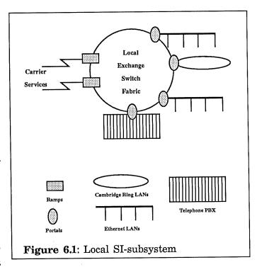
entities that control the site's resources and communicate with peer management entities at remote sites. A typical SI-subsystem, illustrated in Figure 6.1, consists of a local exchange and the collection of ramps, portals, and management systems that are attached to it. The site interconnection service is offered at SI-SAPs which are logically embedded within the individual portals.
