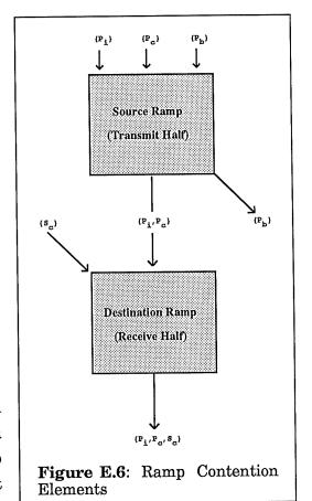
the traffic of interest;  $P_c$ , representing parallel contention traffic mapped to the same channel as  $P_i$ ; and  $P_b$ , the background traffic that is present at the transmit half but mapped to other channels concurrently supported by the transmit half. The secondary input  $S_c$ , which is present at the receive half, represents traffic arriving on other channels concurrently supported by the receive half.<sup>2</sup>
