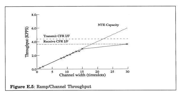
need not be an integer and the predicted throughput is directly proportional to the number of timeslots allocated to the channel.
