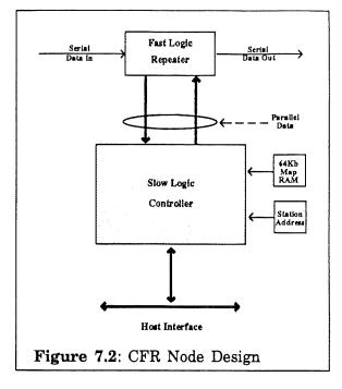
mode the controller is used to create and maintain the ring slot structure, to monitor ring operation, and to receive maintenance information from other nodes.
