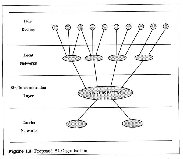
layer. The site interconnection layer (SI-layer), inserted between the local and carrier layers, facilitates communication between peer local networks. This layer is composed of independent subsystems that offer the site interconnection service (SI-service) to their upper layer clients. The subsystems within the SI-layer incorporate management components that facilitate addressing, routing, bandwidth management, security, accounting, etc.
