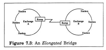
end of the channel presents the incoming packets to its controller, which injects the packets into the peer site's CFR. These ramp-supported bridges support the direct exchange of packets between peer portals attached to different exchanges. So long as the address lists within the bridge mode controllers are correctly configured, packets will flow between sites with minimal in-band intervention.
