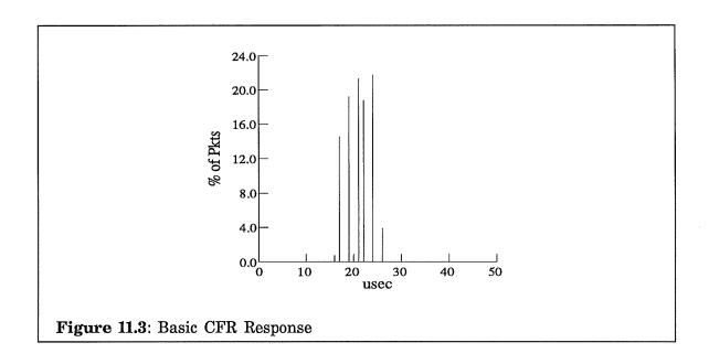
The maximum throughput between stations is limited by this basic response and by the packet loading and unloading times at the peer portals and ramps. In practice, it is the individual stations, in particular the ramps, that determine the packet transfer rate. These results are consistent with the overview of slotted ring performance, presented in Appendix A, and the detailed CFR model developed in Appendix D.
