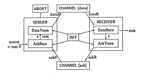
Figure 9: HOL Sliding Window Protocol Model
