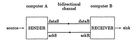
Figure 5: Physical environment for a sliding window protocol
