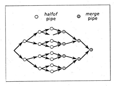
Figure 5.7: Concurrent structure of mergesort
