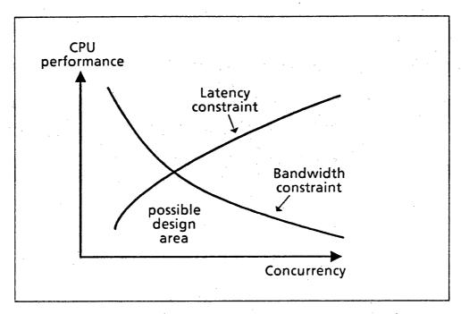
Figure 4.1: Latency and Bandwidth Constraints on CPU performance
