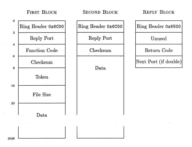
Figure 7.2: Block Formats for Single and Double Block Transfers
