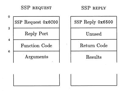
Figure 6.1: Basic Block Formats for the Single Shot Protocol
