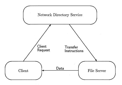
Figure 5.1: Critical Path for Fetching Data
