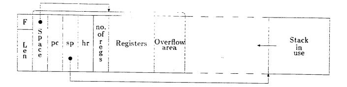
Figure 3: Format of a Stack Segment.
