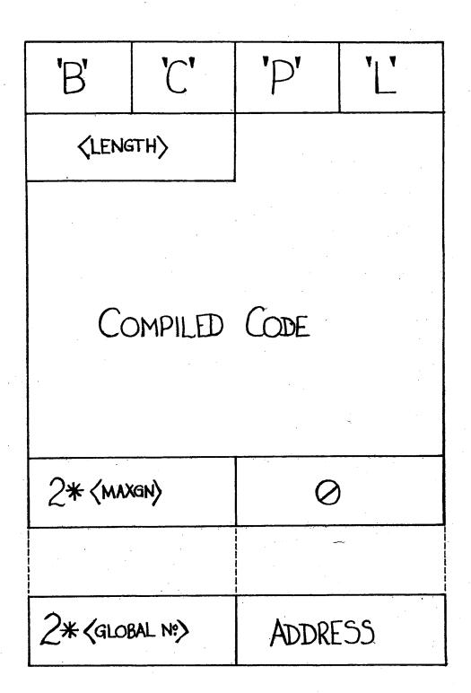
Fig. B.3.1 The layout of a BCPL module
