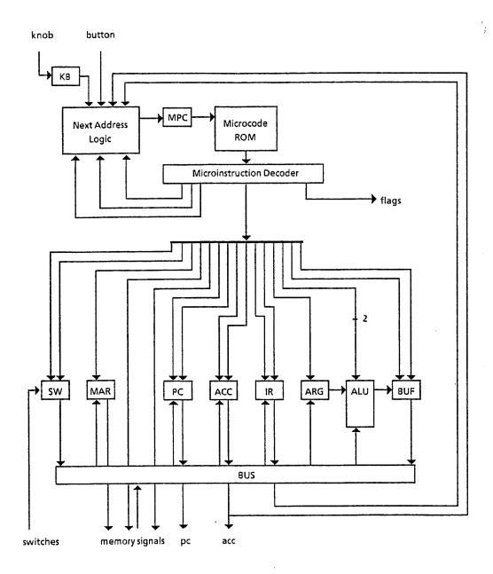
Figure 4: Register-Transfer Level Architecture.
