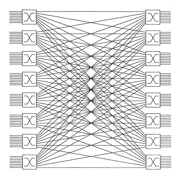
Fig. 2. A 64×64 delta network of 8×8 switching elements
