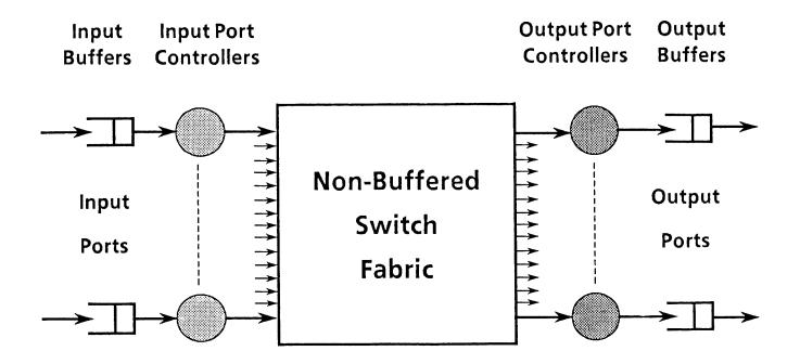
Fig. 1. Basic structure of the fast packet switch
