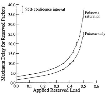
Fig. 11. Maximum reserved service packet delay for the Poisson reserved service traffic model with and without saturated unreserved service traffic
