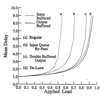
Fig. 7. Mean delay performance of crossbar switch fabrics for slotted traffic
