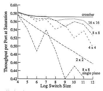
Fig. 8. Throughput at saturation for single plane, pure input buffered, flooding delta networks
