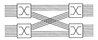
Fig. 3. A 16×16 modified delta network of 8×8 switching elements
