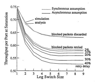
Fig. 6. Throughput at saturation for the crossbar switch
