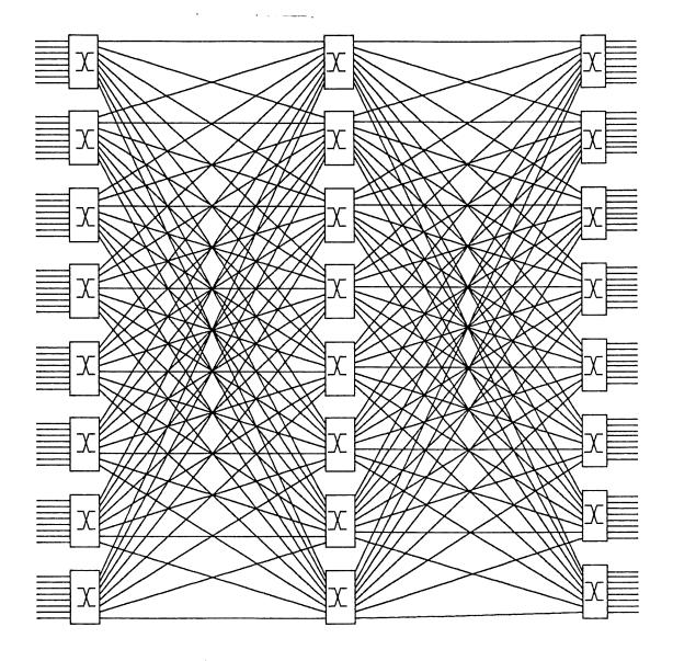
Fig. 4. A 64×64 Beneš network of 8×8 switching elements
