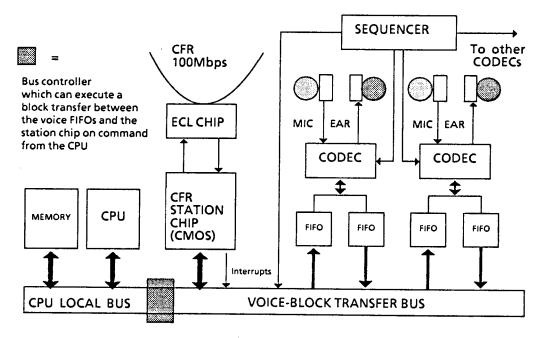
Figure 4.4: A Cambridge Fast Ring (CFR) telephone
