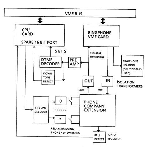
Figure 4.6: A block diagram of the ISLAND gateway
