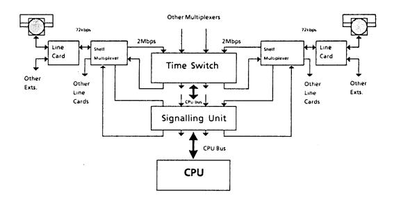
Figure 2.1: Schematic of a first generation line shelf PABX
