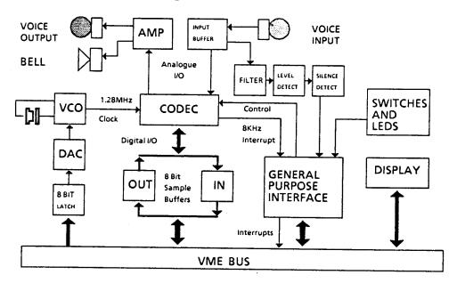
Figure 4.3: The essential components of the ISLAND Ringphone
