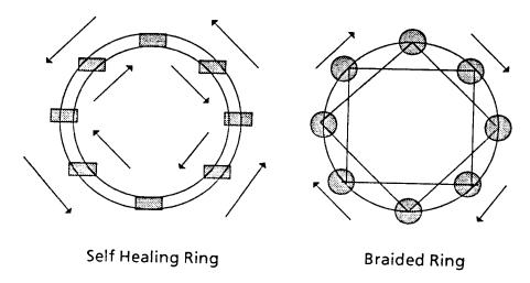
Figure 3.2: Two types of fault tolerant ring network
