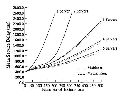
Figure 9.6: A Comparison of Multicast against a Virtual Ring protocol
