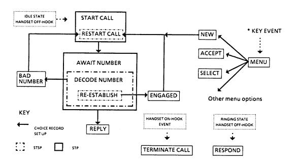
Figure 5.2: The ISLAND Call Finite State Machine (CFSM)
