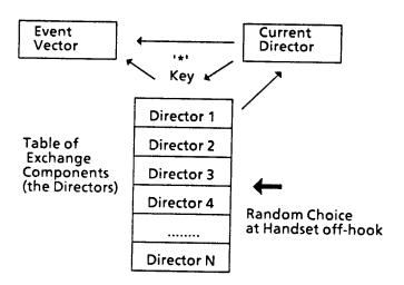
Figure 4.2: A mechanism for finding a controller
