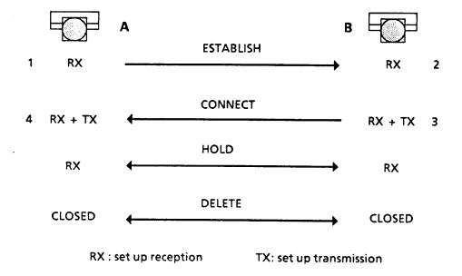
Figure 5.4: Using the ECHD interface to set up a voice connection
