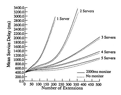
Figure 9.2: Service delays when using a 2000ms monitor probe
